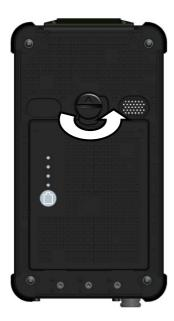
Turn counterclockwise with a slot screwdriver or a coin to unlock the Battery Lock, and then replace the battery.
