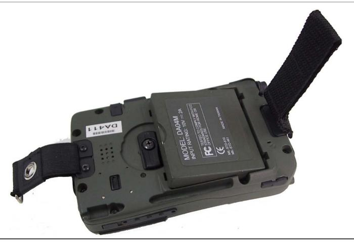
Note: During battery swap the memory data is sustained by a small backup battery. Please swap battery within 1 minute to avoid data loss.
