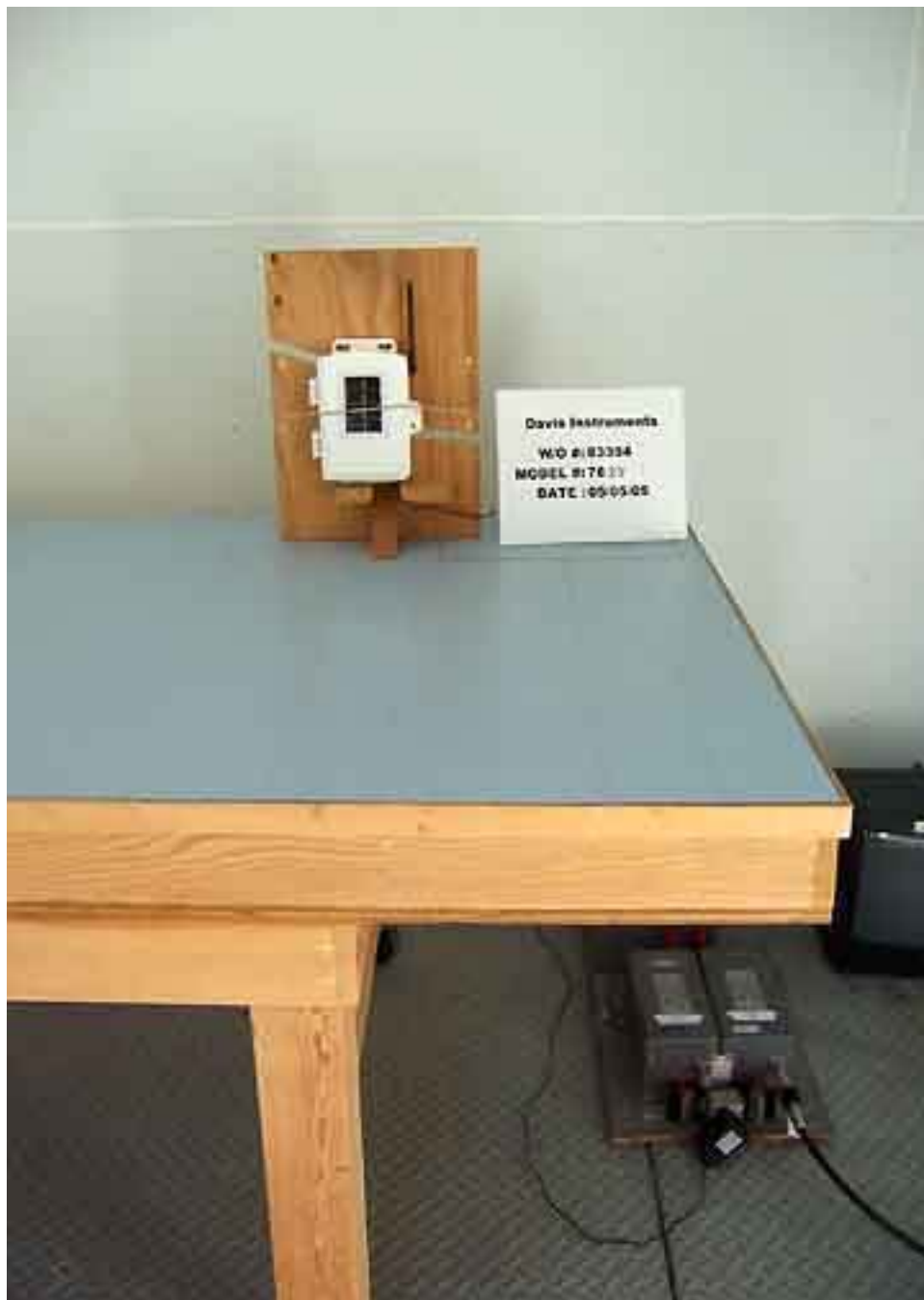
Mains Conducted Emissions - Front View
