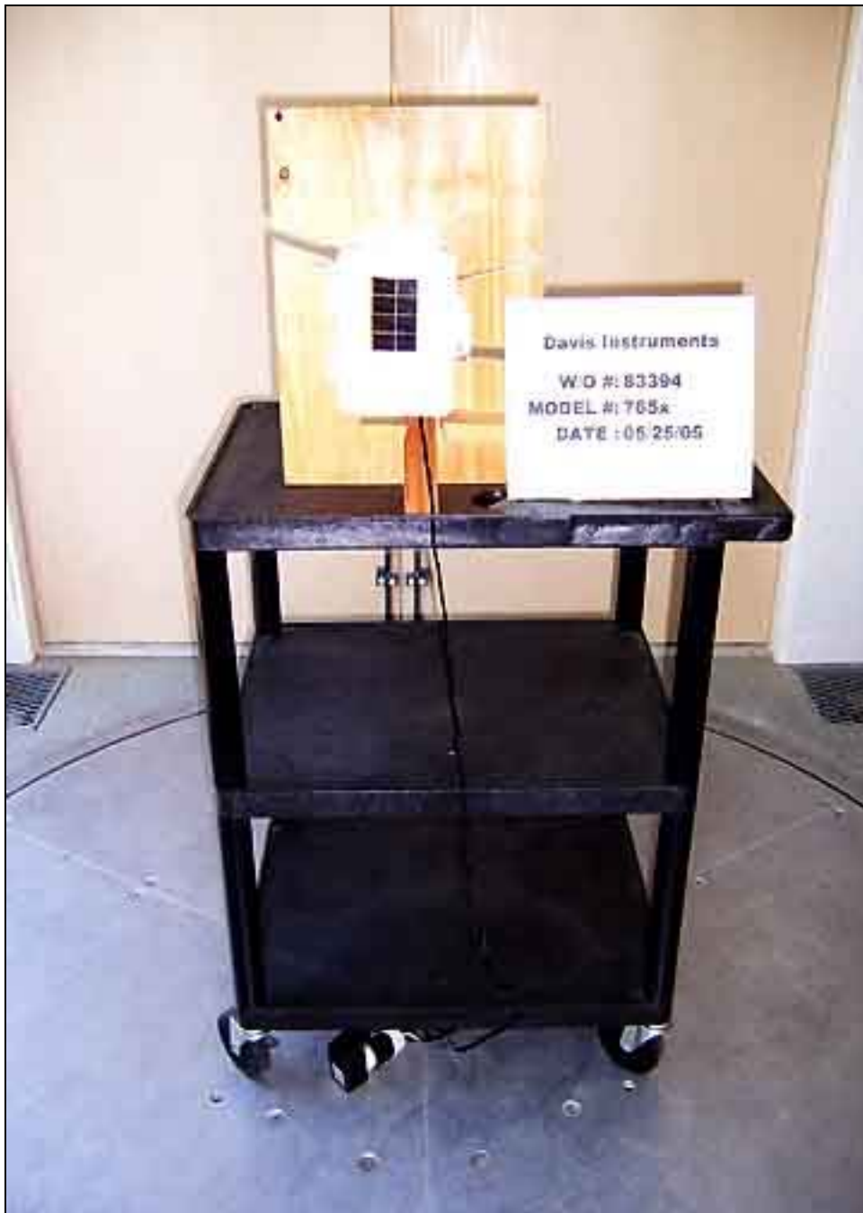
Radiated Emissions - Receiver
