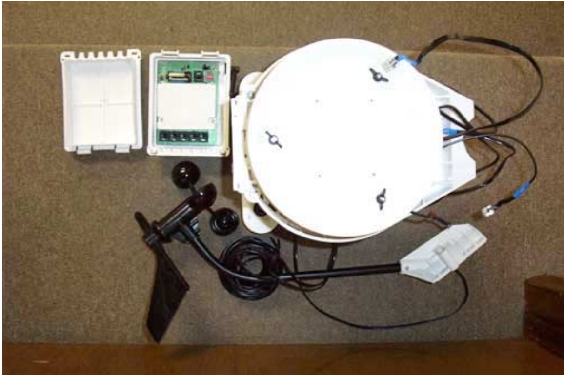
PCB Enclosure Removed from Weather Station
