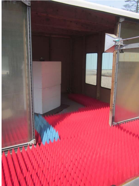
Horizontal Antenna Polarization, 1 GHz to 18 GHz, Double Ridge Guide
