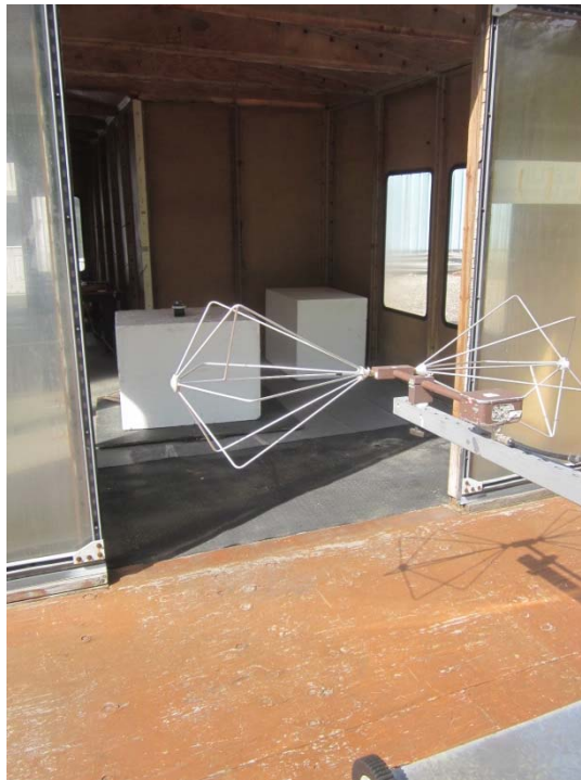
Horizontal Antenna Polarization, 30 MHz to 200 MHz, Biconical Antenna
