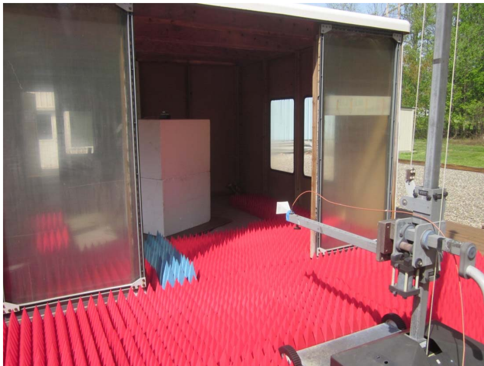
Vertical Antenna Polarization, 18 GHz to 25 GHz, Horn
