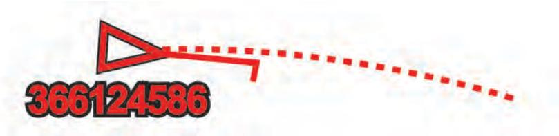
When course over ground and heading information are provided by an activated AIS target, but rate of turn information is not provided, the projected course of the target is calculated based on the course over ground information.
