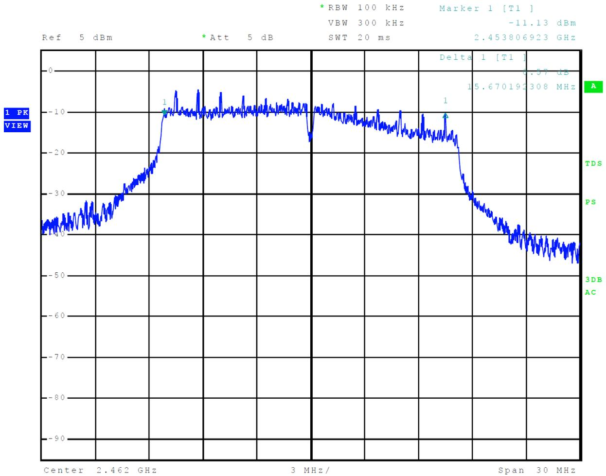
**Figure 13 Plot of 99% Occupied Bandwidth Mode 4 802.11g**
