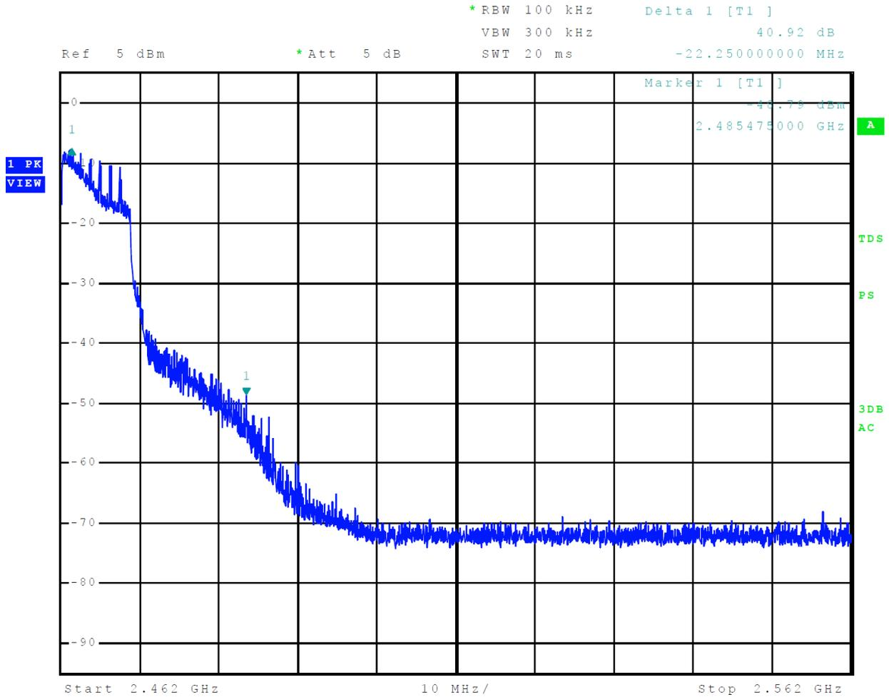
**Figure 10 Plot of 6-dB Occupied Bandwidth Mode 3 802.11b**
