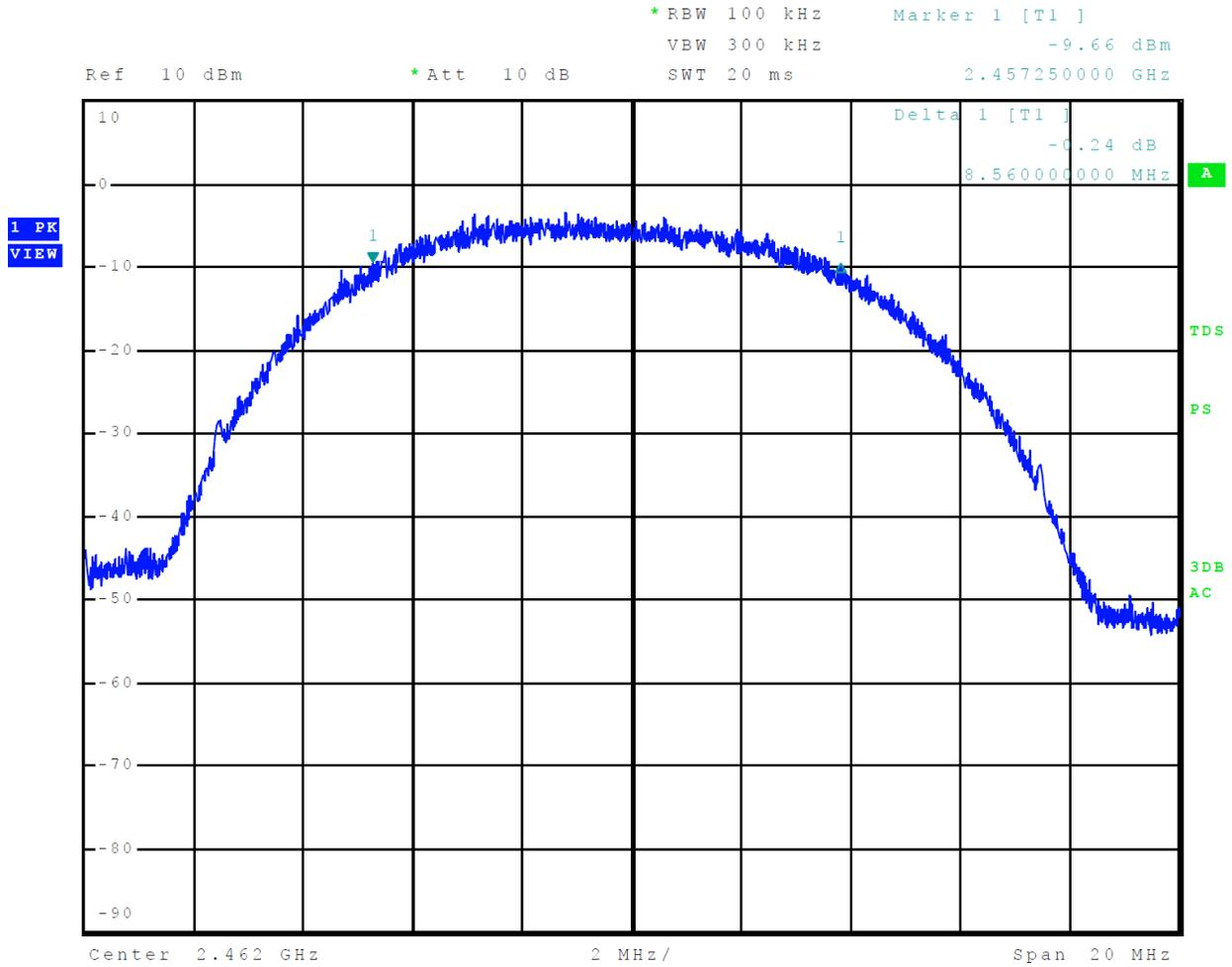
Figure 11 Plot of 99% Occupied Bandwidth Mode 3 802.11b
