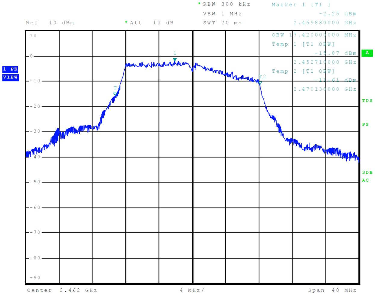
Figure 14 Plot of 6-dB Occupied Bandwidth Mode 5 802.11n
