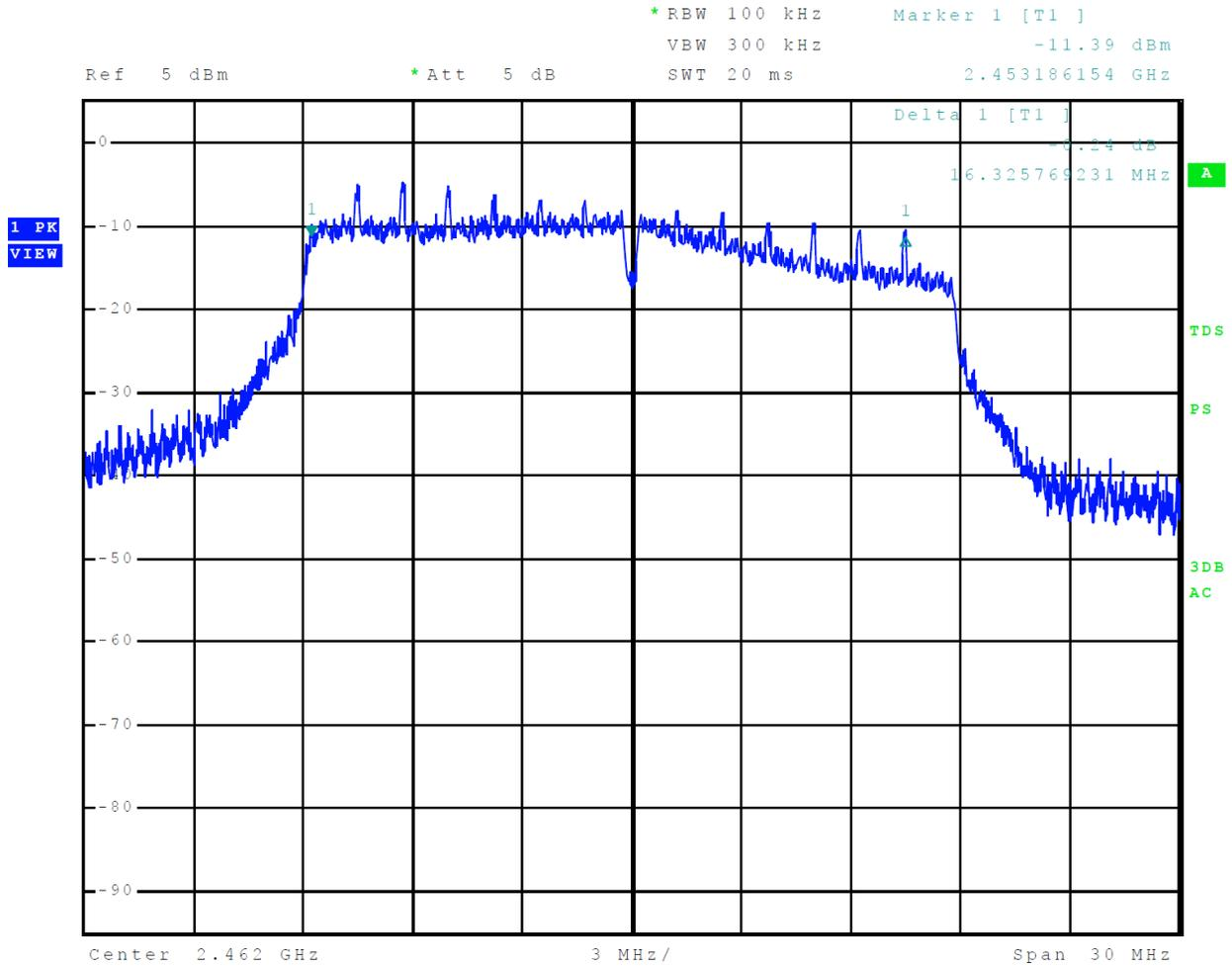
Figure 15 Plot of 99% Occupied Bandwidth Mode 5 802.11n
