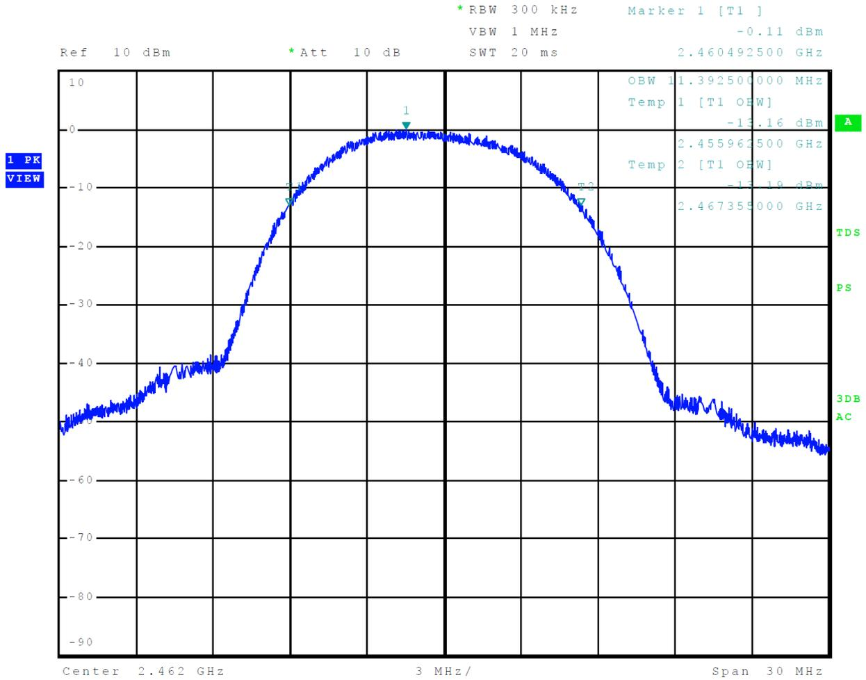
Figure 12 Plot of 6-dB Occupied Bandwidth Mode 4 802.11g
