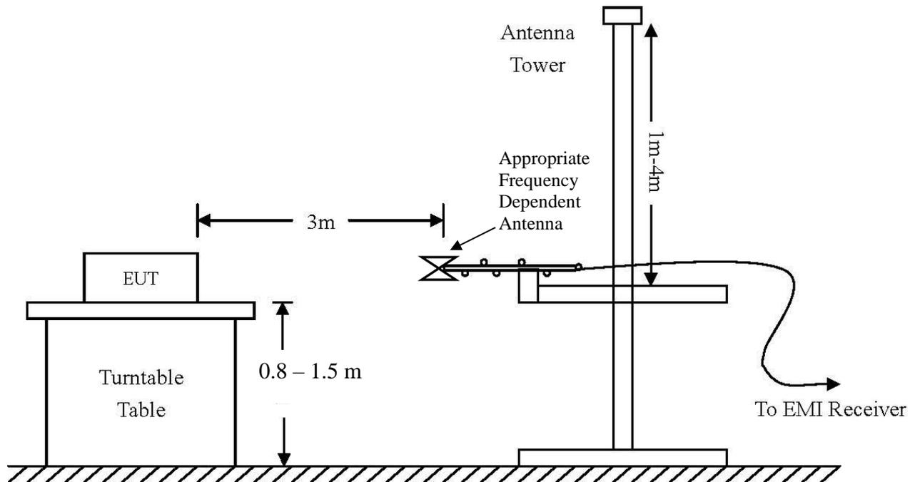
**Diagram 3 Test arrangement for Antenna Port Conducted emissions**
