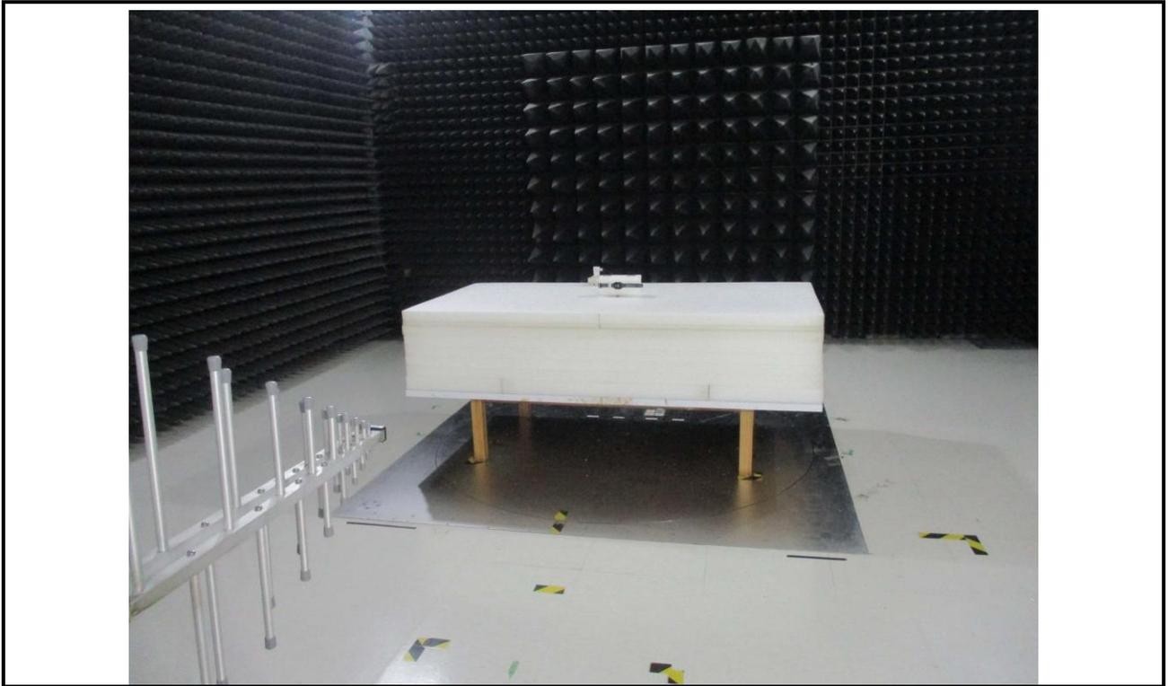
**Radiated Emission Above 1GHz Test**
