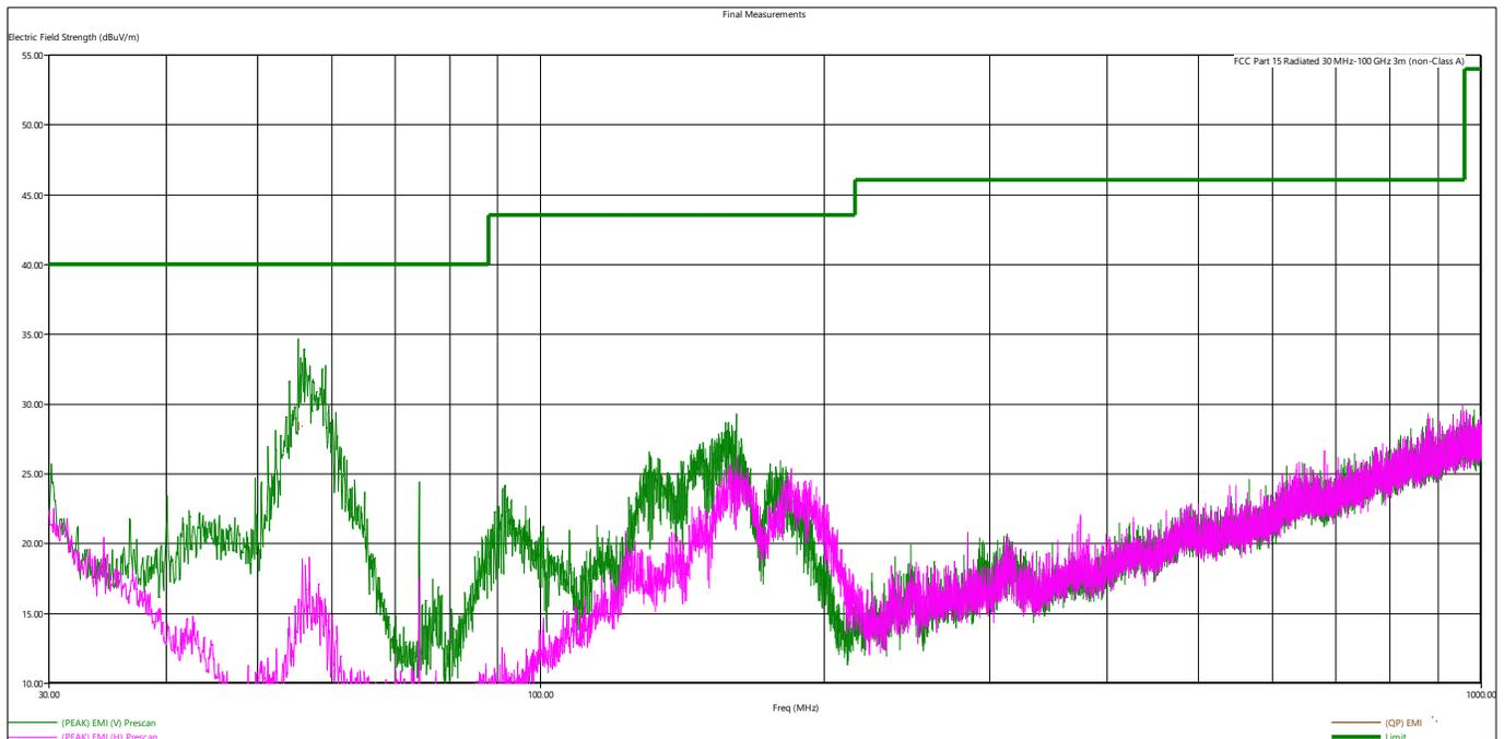
**Figure 5 - Radiated Emissions Plot, 802.11b**
