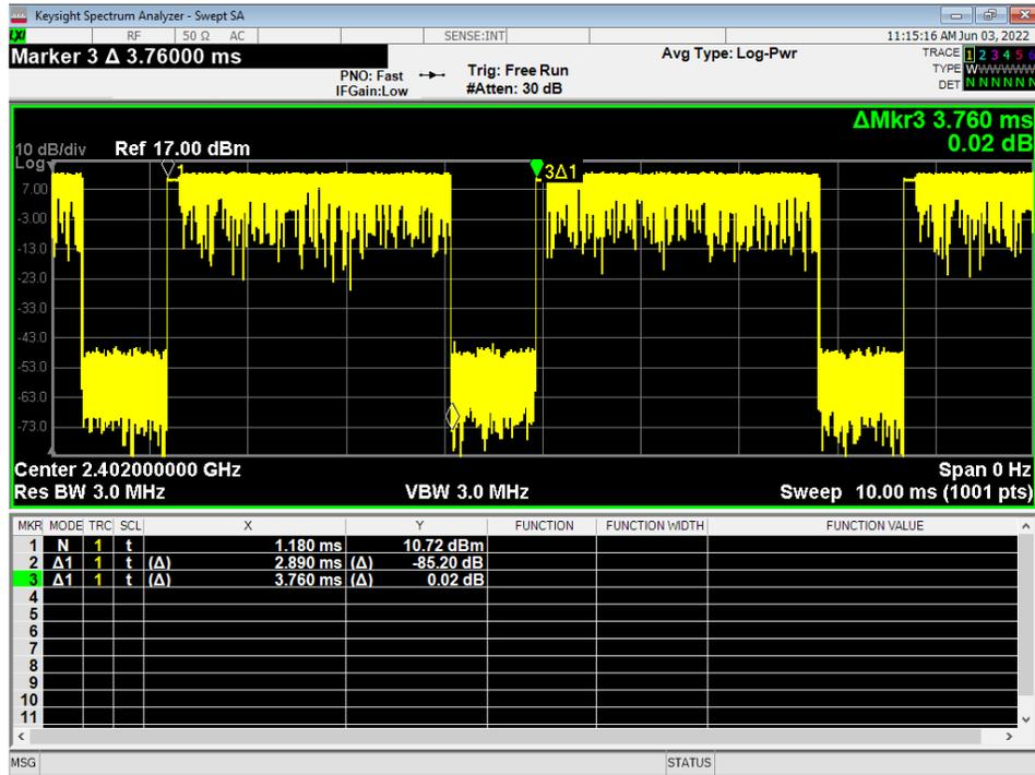
Figure 4 – 3EDR Duty Cycle
