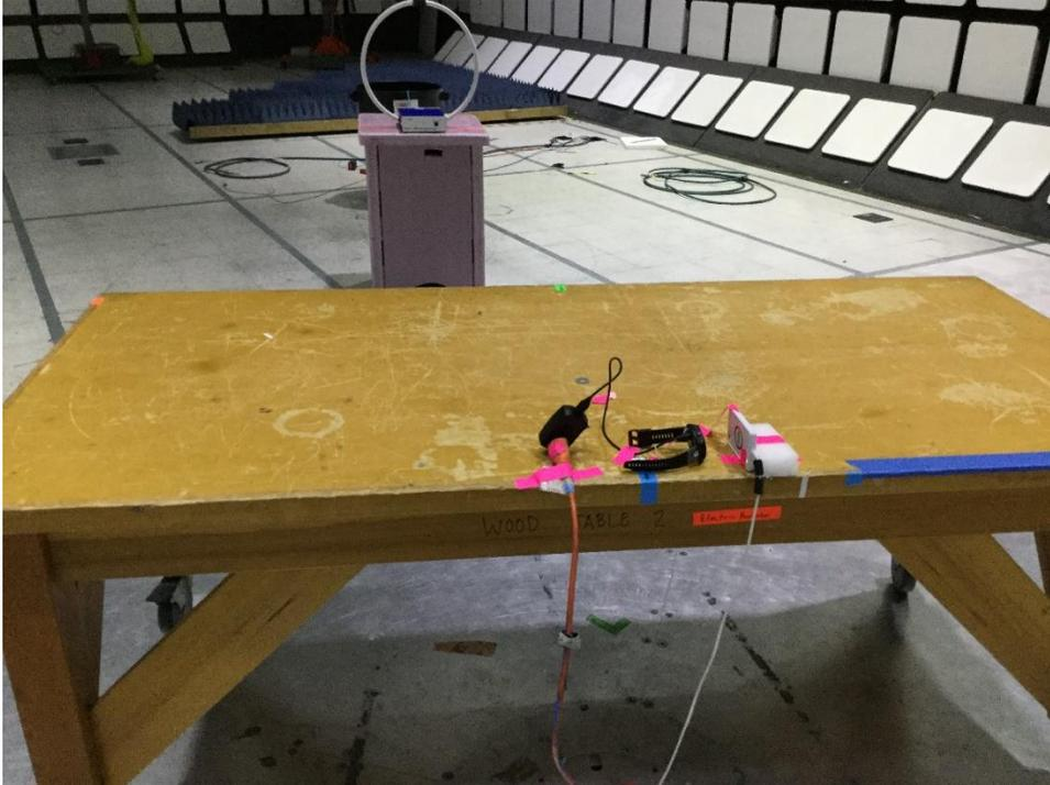
10M – 30 MHz test setup
