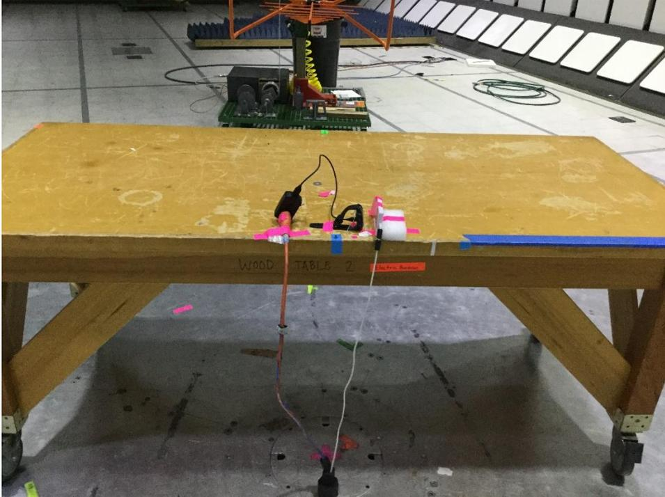
30 MHz – 1 GHz Test Setup, NFC
