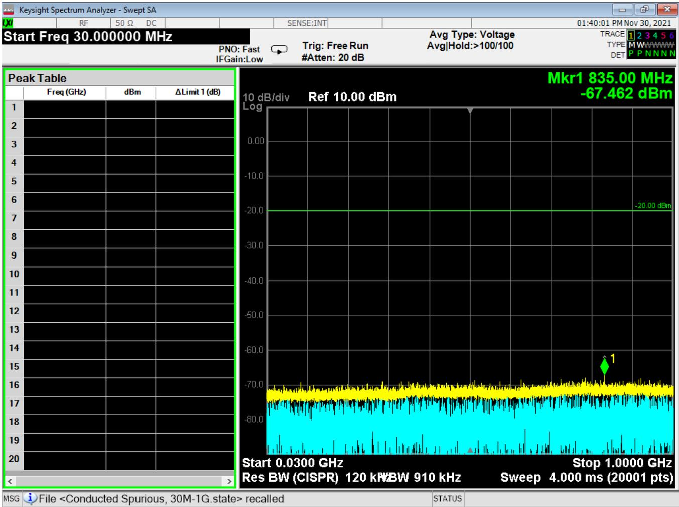
Figure 8 - Radiated Emissions Plot, WIFI 802.11b, 30M – 1G
