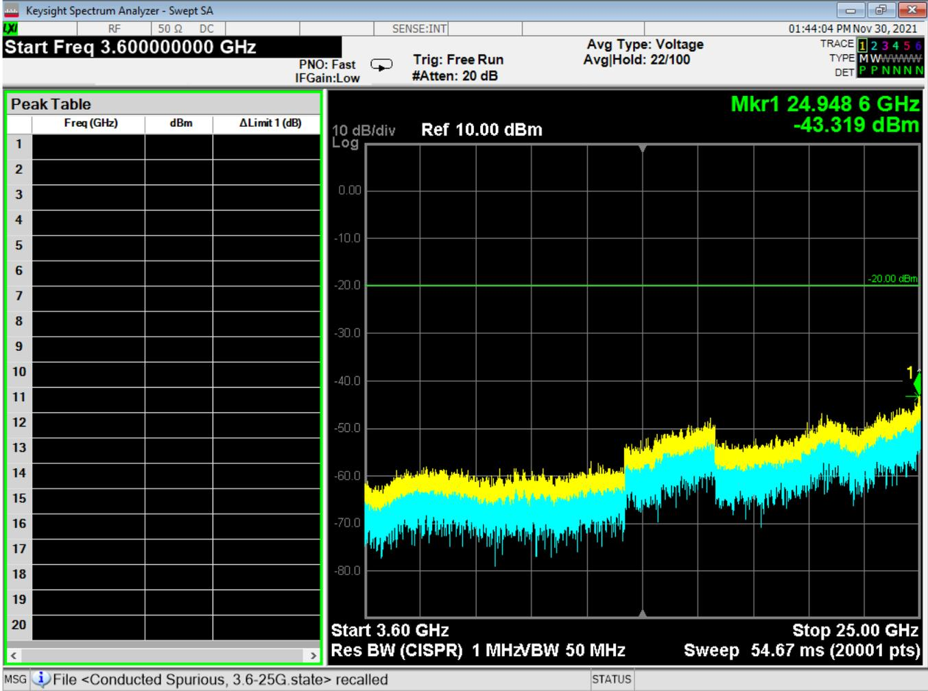
Figure 16 - Radiated Emissions Plot, WIFI 802.11n, 3.6G – 25G
