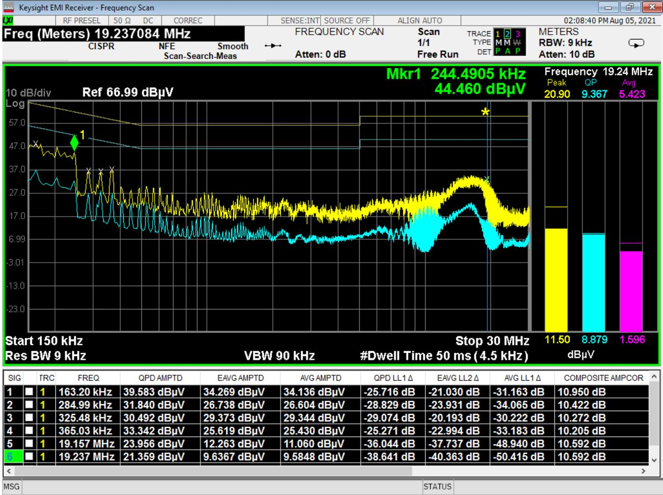
Figure 19 - Conducted Emissions Plot, Line, IDLE
