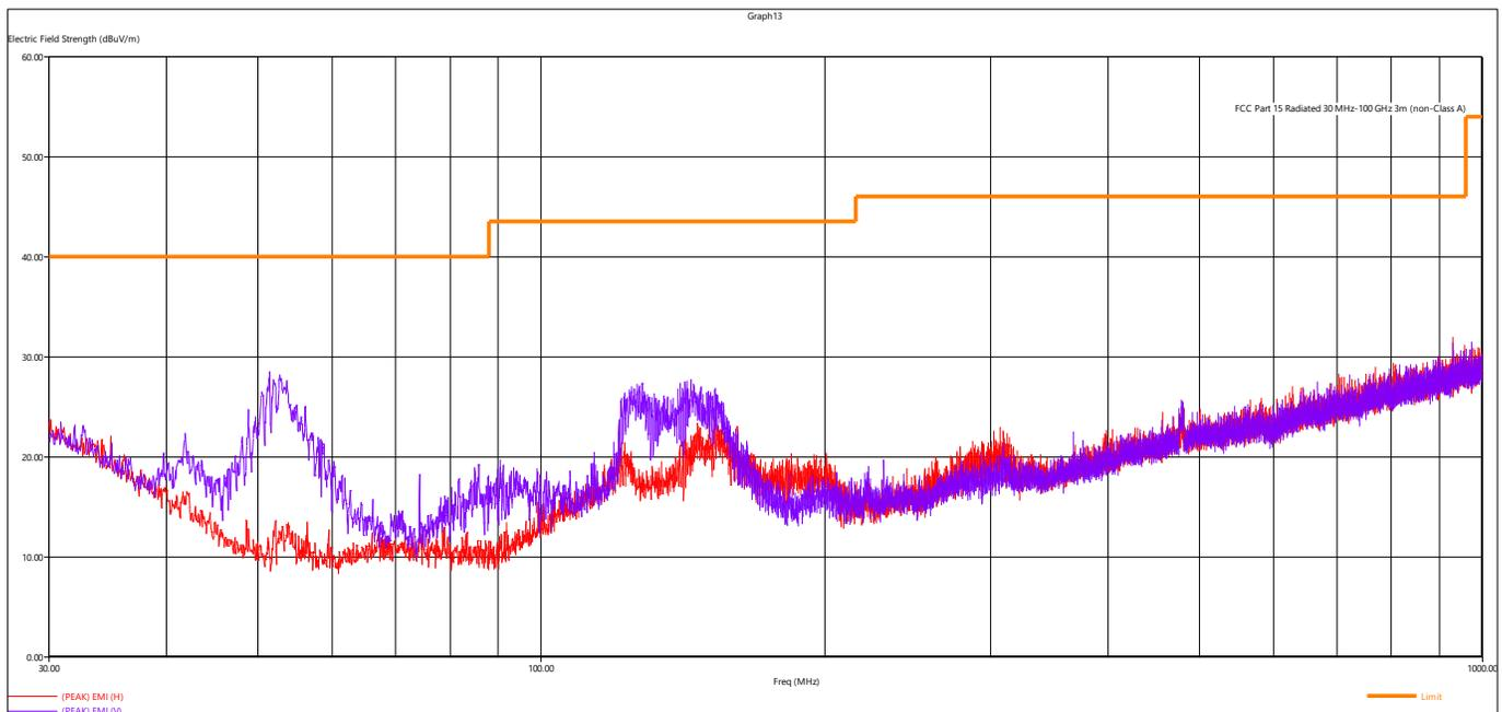
Figure 7 - Radiated Emissions Plot, 802.11n
