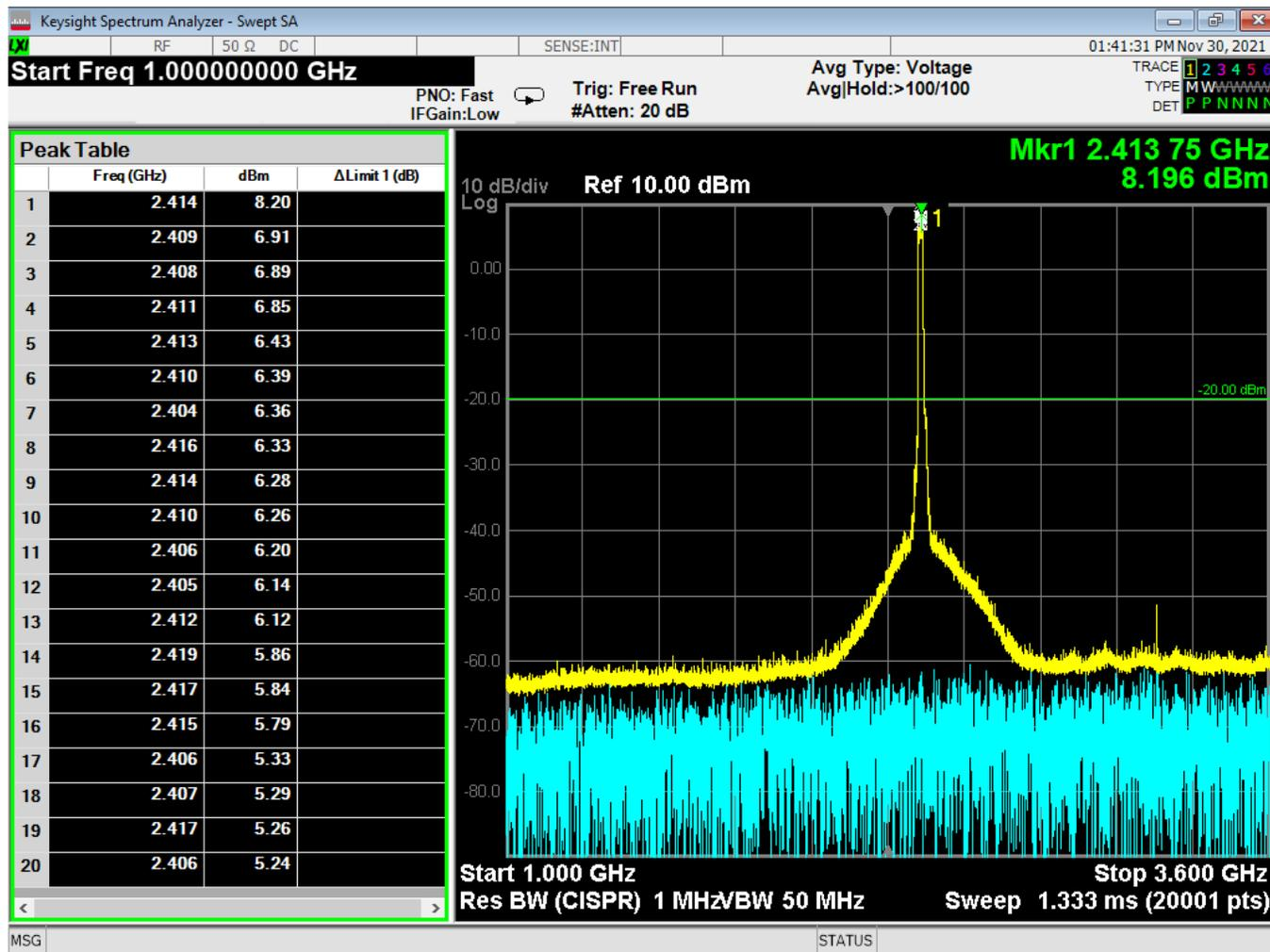
Figure 12 - Radiated Emissions Plot, WIFI 802.11g, 1G – 3.6G
