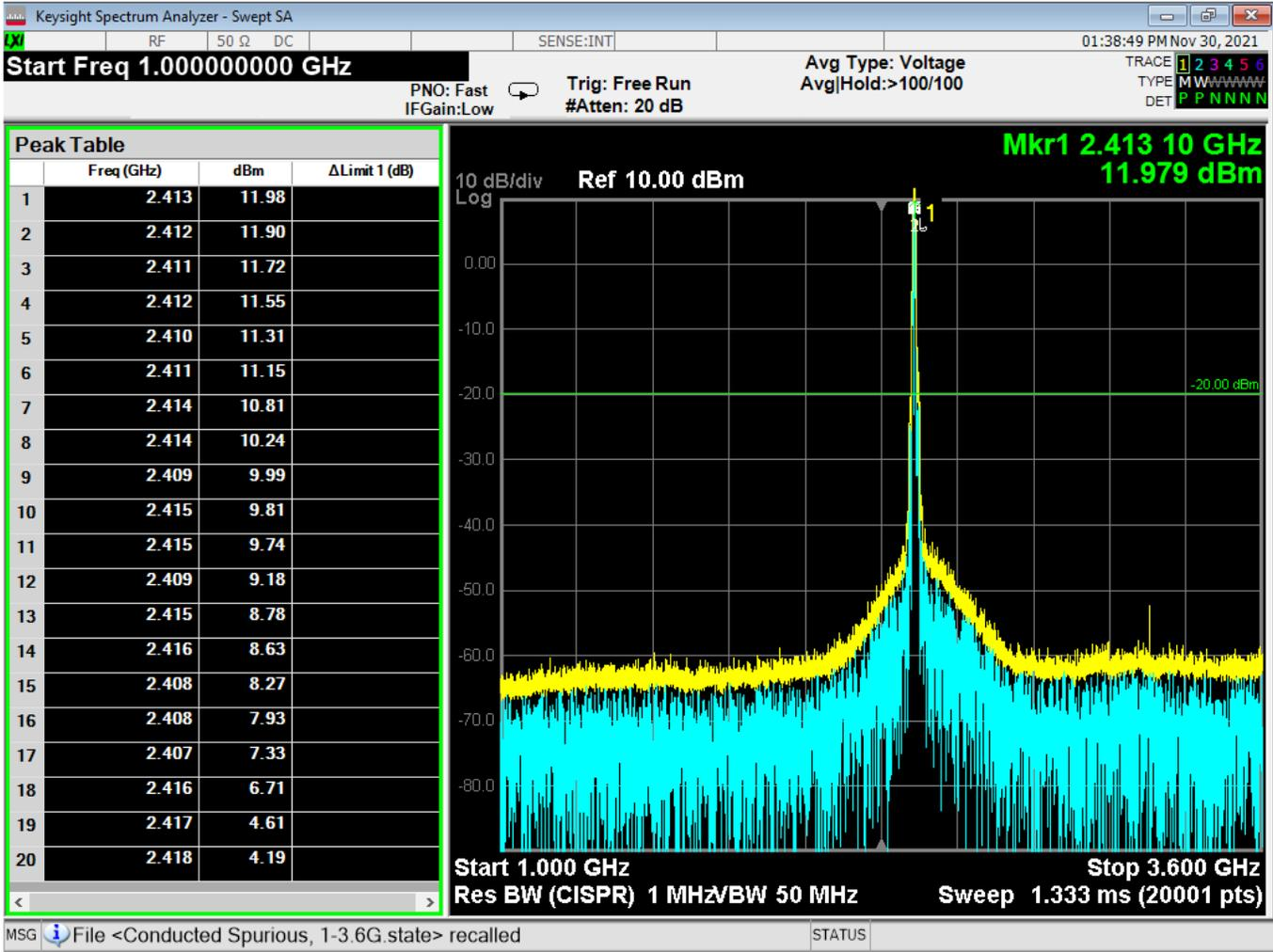
Figure 9 - Radiated Emissions Plot, WIFI 802.11b, 1G – 3.6G
