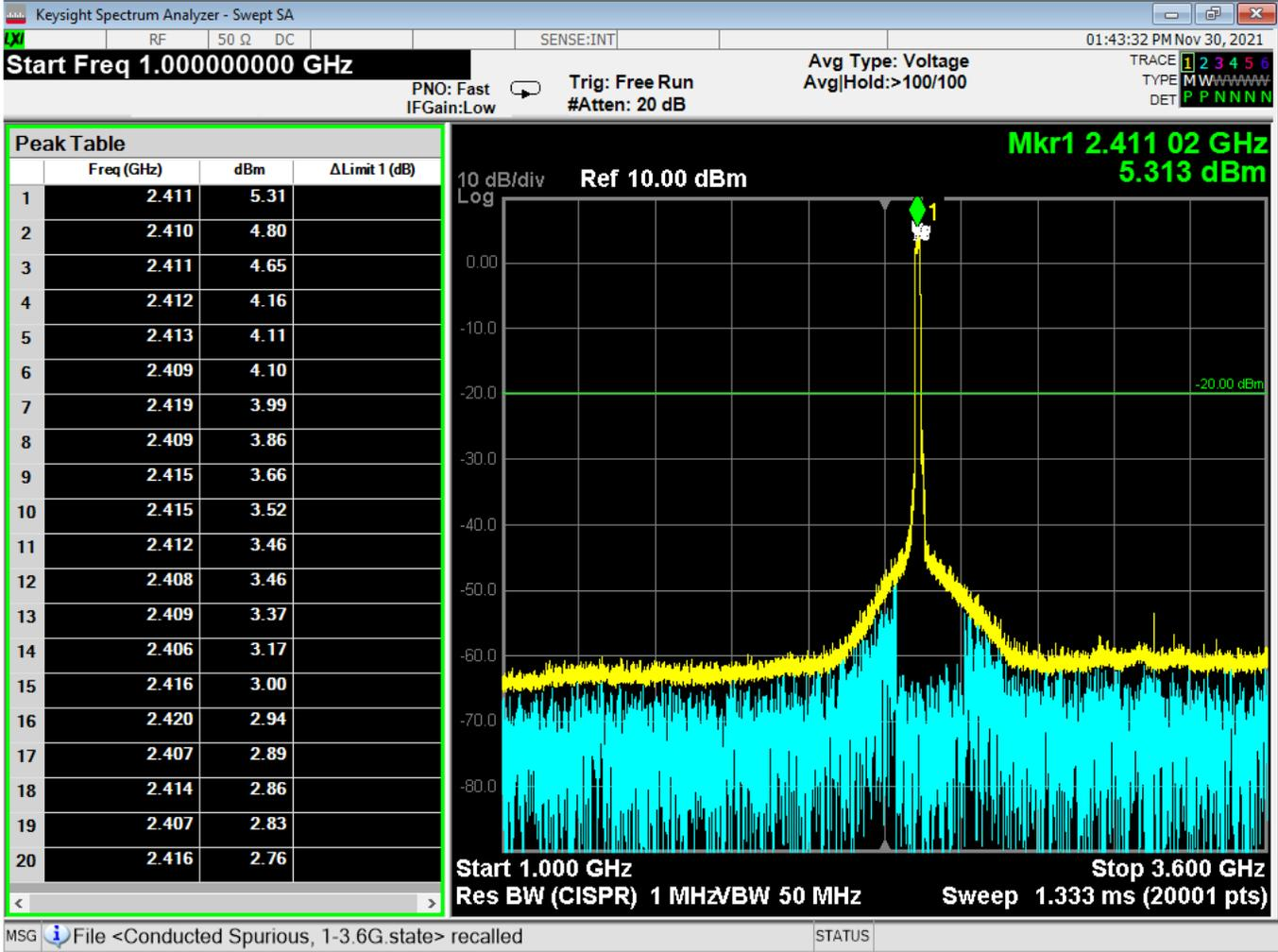
Figure 15 - Radiated Emissions Plot, WIFI 802.11n, 1G – 3.6G
