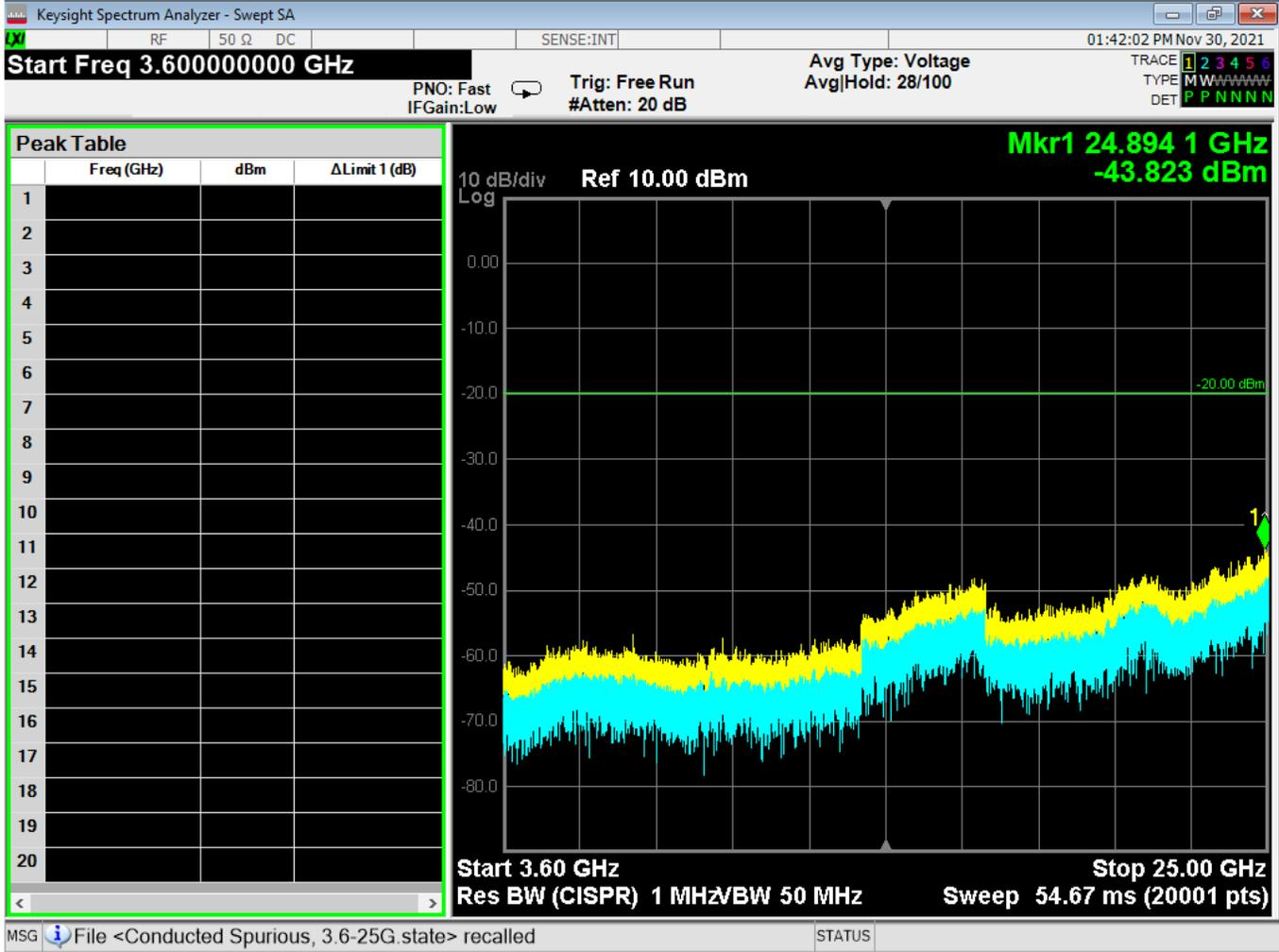
Figure 13 - Radiated Emissions Plot, WIFI 802.11g, 3.6G – 25G
