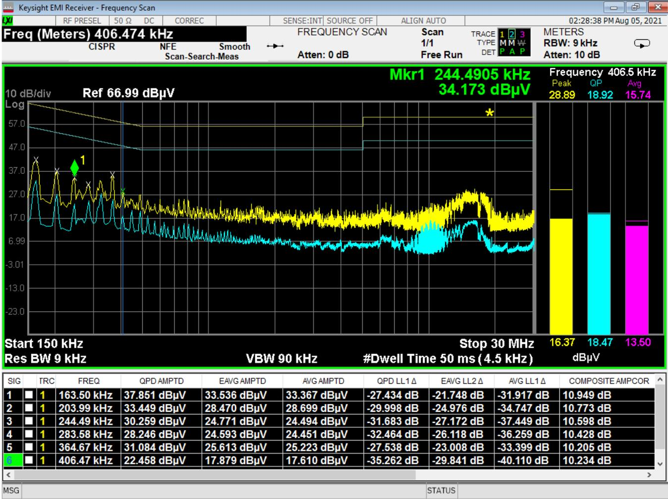
Figure 18 - Conducted Emissions Plot, Neutral, TX
