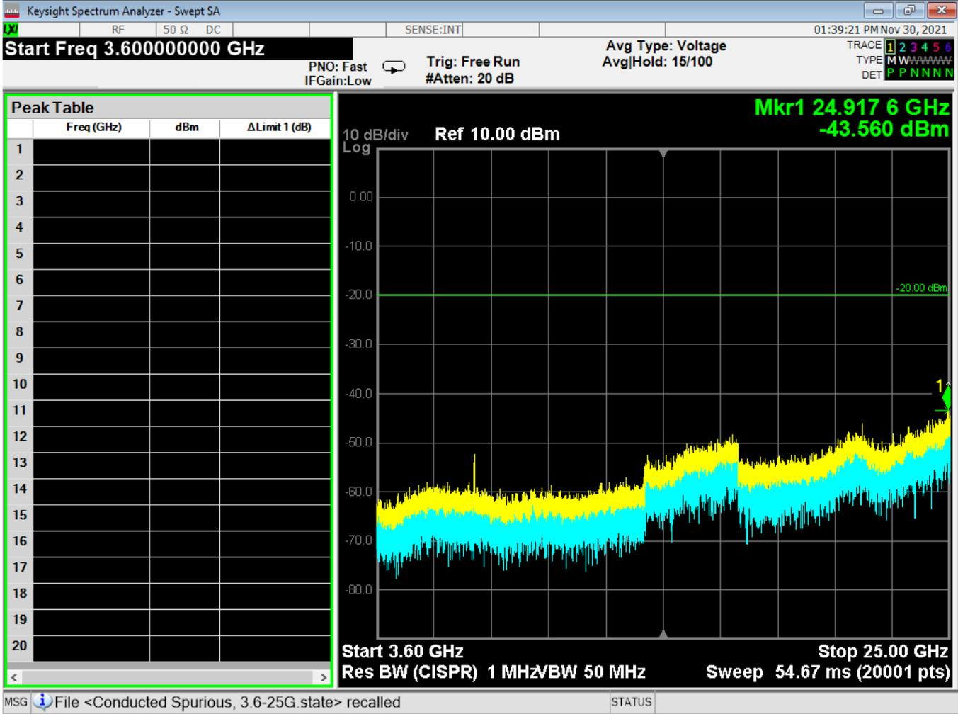
Figure 10 - Radiated Emissions Plot, WIFI 802.11b, 3.6G – 25G
