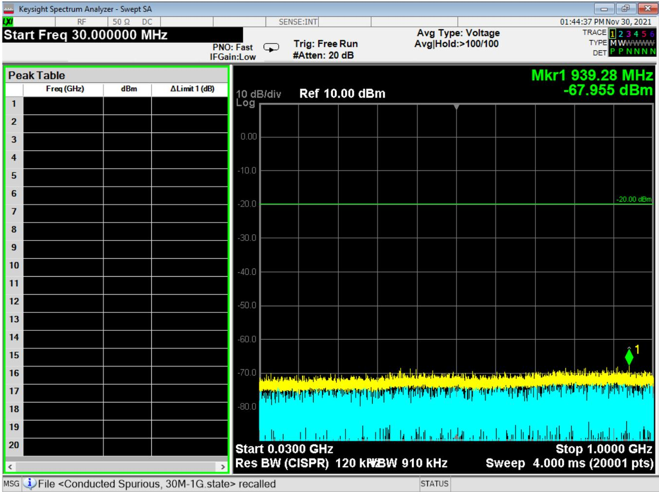
Figure 14 - Radiated Emissions Plot, WIFI 802.11n, 30M – 1G
