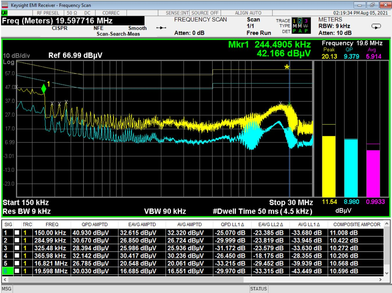
Figure 15 - Conducted Emissions Plot, Line, TX
