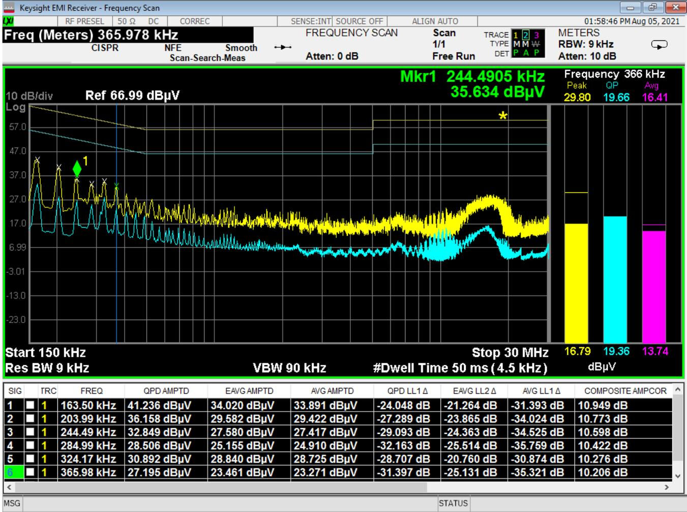
Figure 18 - Conducted Emissions Plot, Neutral, IDLE
