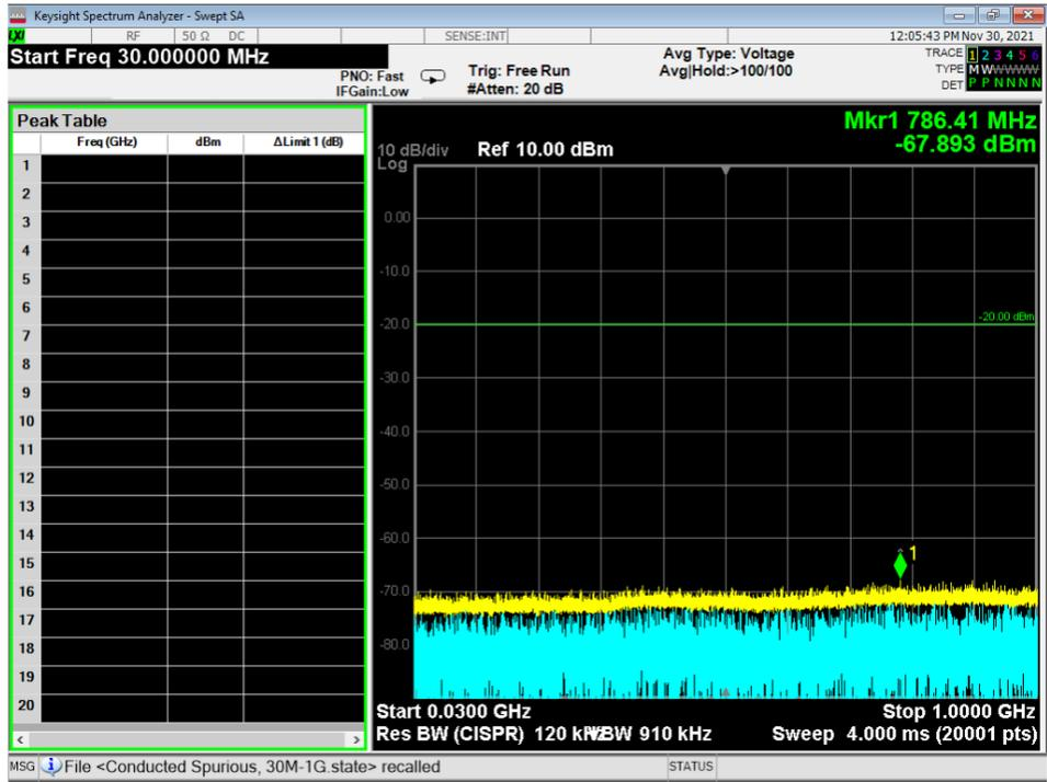
Figure 12 - Radiated Emissions Plot, 3EDR, 30M – 1G
