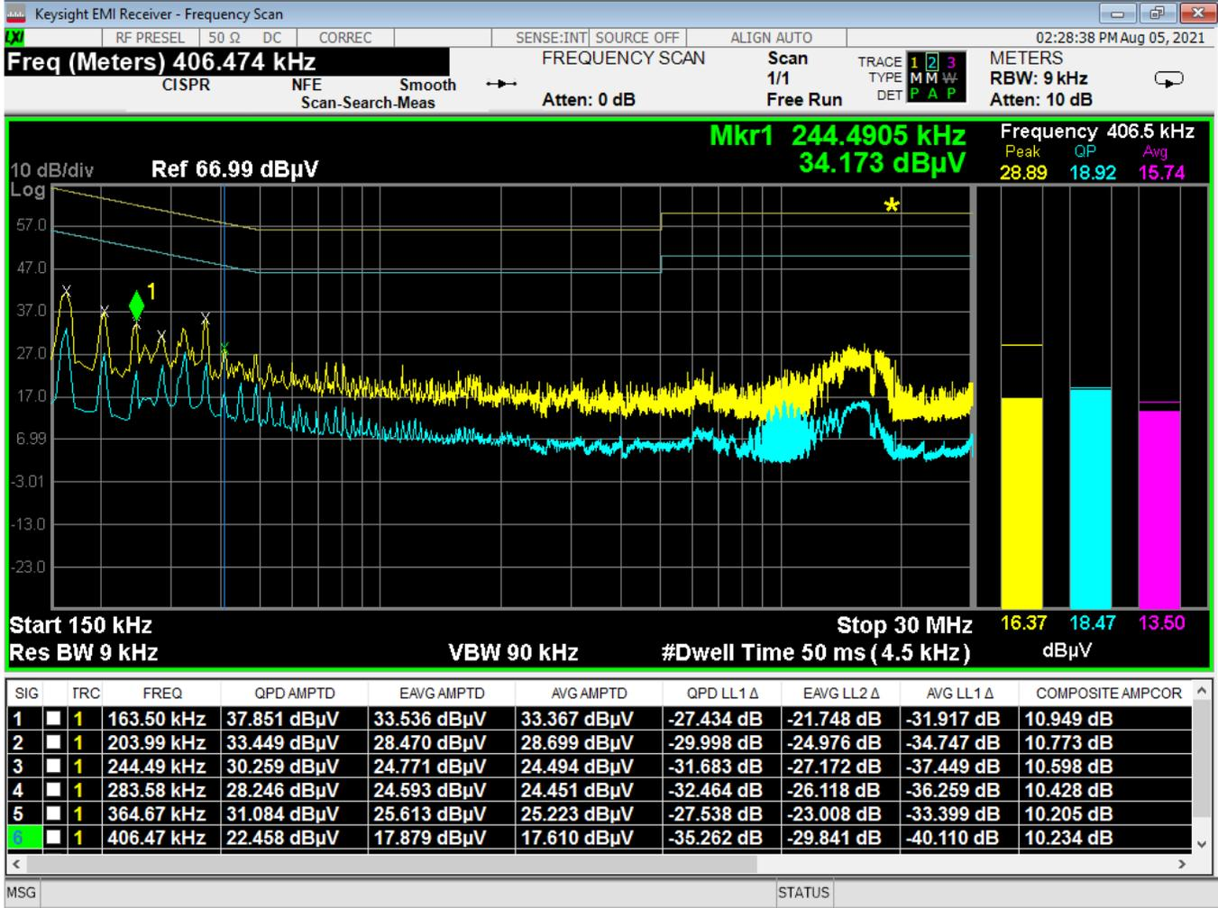
Figure 16 - Conducted Emissions Plot, Neutral, TX
