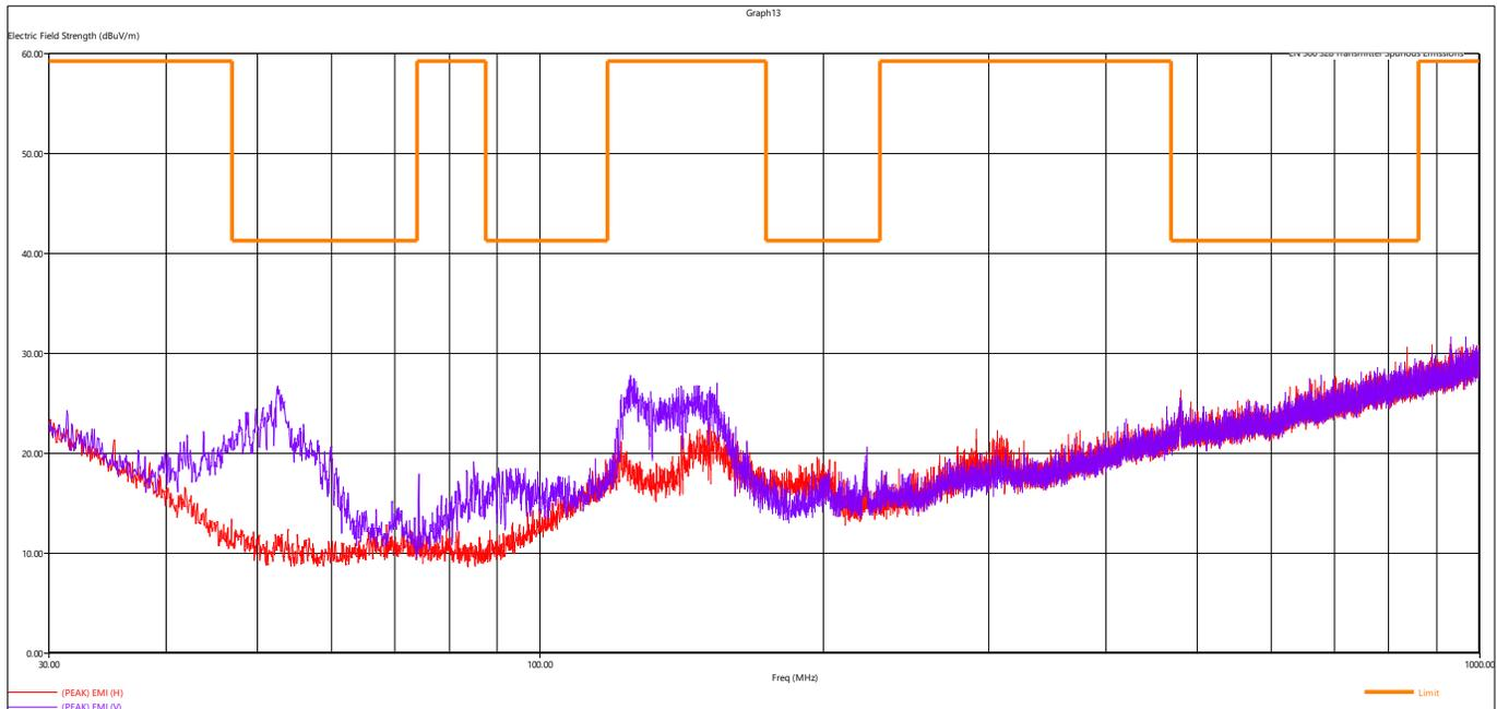
Figure 8 - Radiated Emissions Plot, BT EDR 3MB
