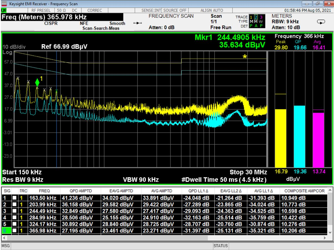
Figure 13 - Conducted Emissions Plot, Neutral, IDLE
