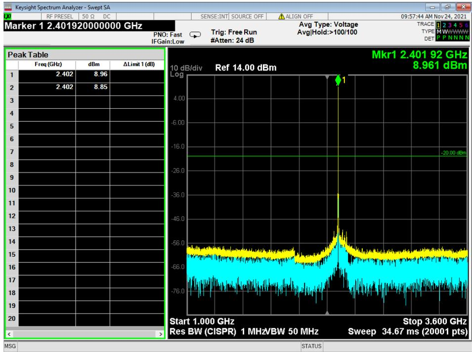
Figure 7 - Radiated Emissions Plot, BTBR, 1G – 3.6G
