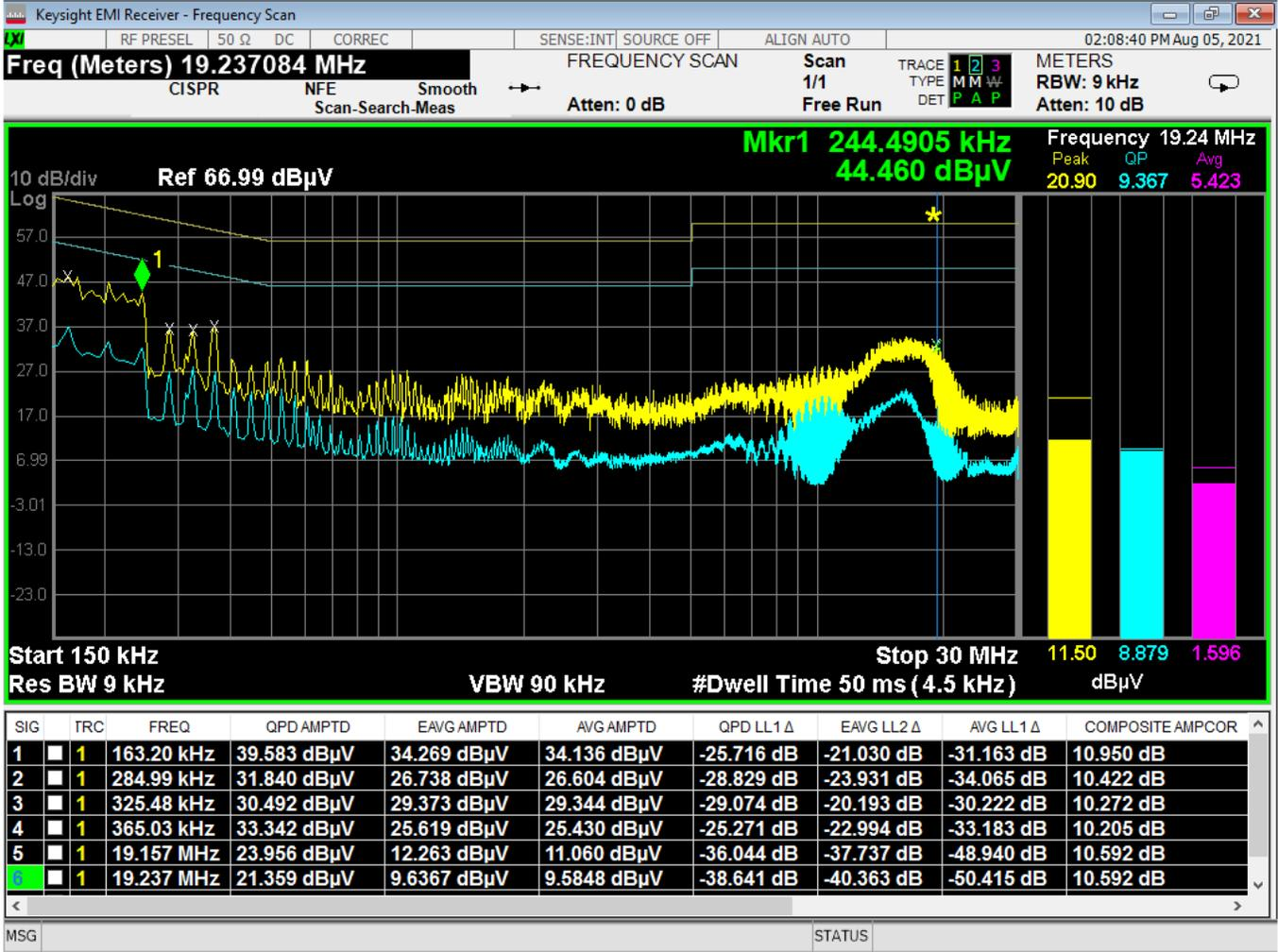
Figure 11 - Conducted Emissions Plot, Line, IDLE
