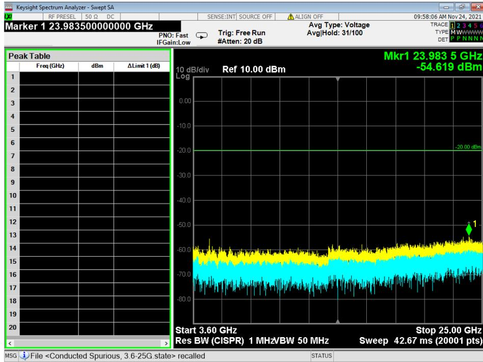
Figure 8 - Radiated Emissions Plot, BTBR, 3.6G – 25G
