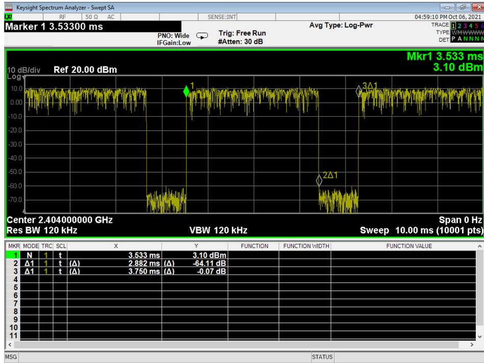
$$\text{DCCF (Duty Cycle Correction Factor)} = 20 * \text{Log}(\text{Duty Cycle} / 100)$$
