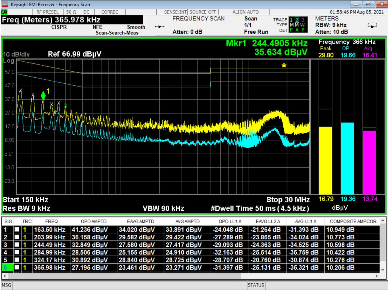
Figure 12 - Conducted Emissions Plot, Neutral, IDLE
