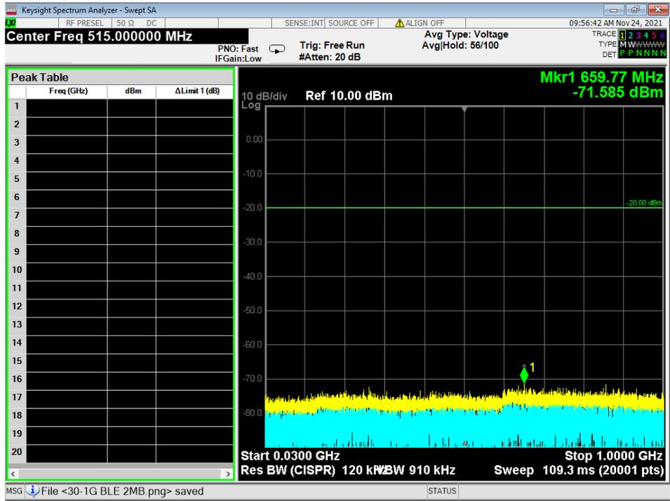
Figure 6 - Radiated Emissions Plot, BTBR, 30M – 1G
