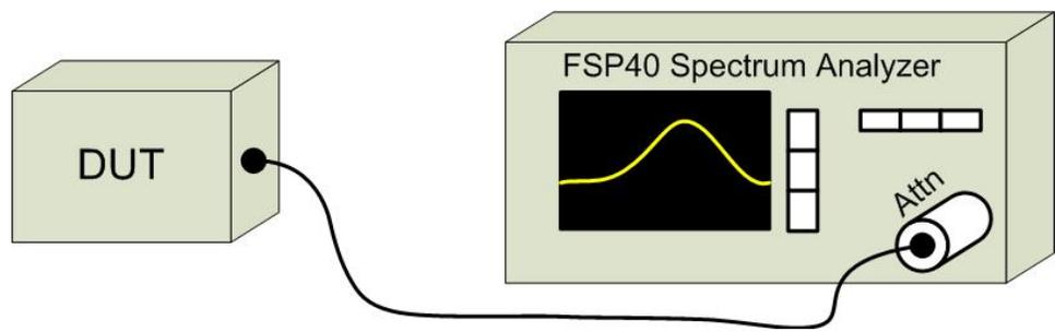
**Table A.2 – Radiated Emissions Measurement Equipment**
