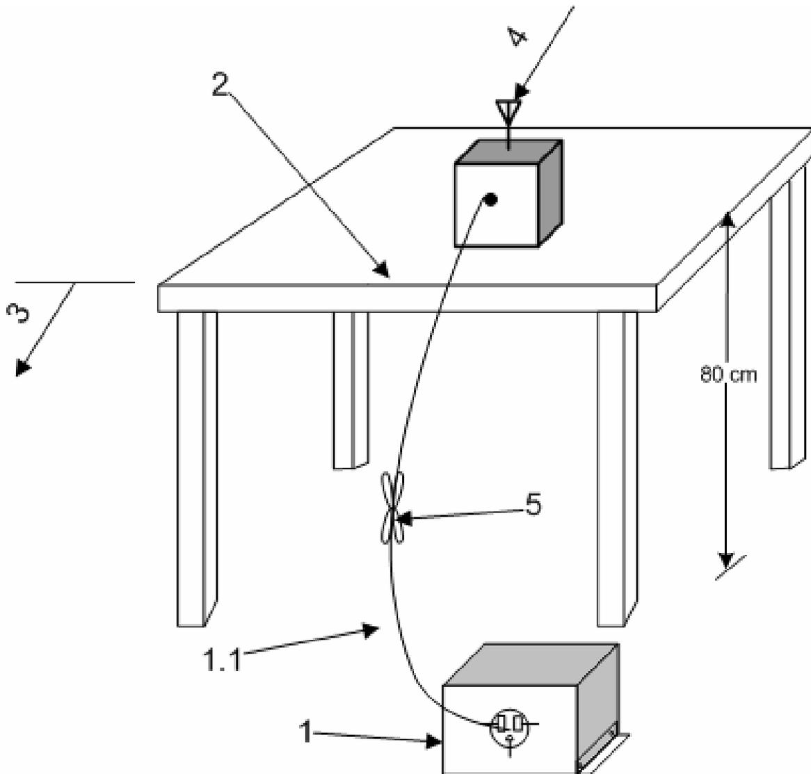
1—A LISN is optional for radiated measurements between 30 MHz and 1000 MHz but not allowed for measurements below 30 MHz and above 1000 MHz (see 6.3.1). If used, then connect EUT to one LISN. Unused LISN measuring port connectors shall be terminated in 50 Ω loads. The LISN may be placed on top of, or immediately beneath, the reference ground plane (see 6.2.2 and 6.2.3.2).
