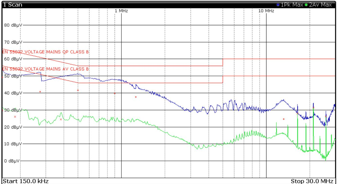
**Table 9 AC Line Conducted Emissions Data L1 (EUT – AC Adapter)**
