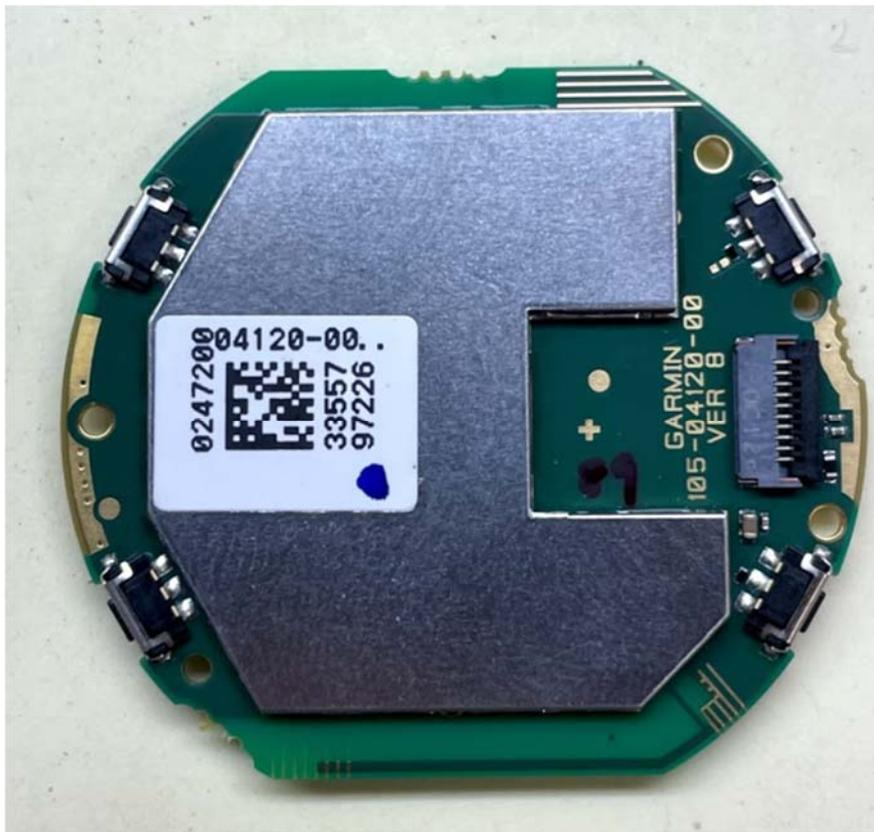
**Figure E19.3 – Internal Photo – PCB Front, Shield Removed**
