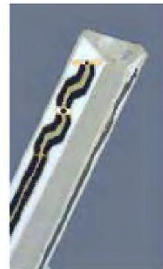
Figure 2.3 Probe Thick-Film Technique
