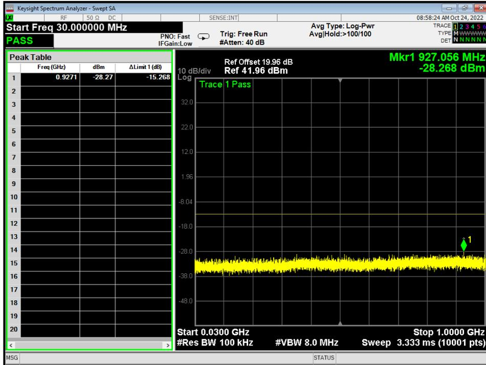
Figure 14 - Conducted Spurious Plot, 30M – 1G
