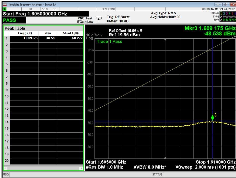
Figure 13 – Part 25.216(g), Transmitting at 1625.979167 MHz, Conducted Measurement
