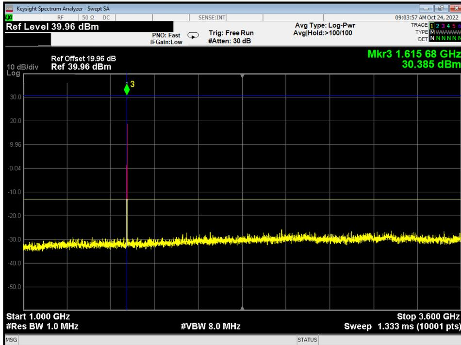
Figure 15 - Conducted Spurious Plot, 1G – 3.6G, Fundamental
