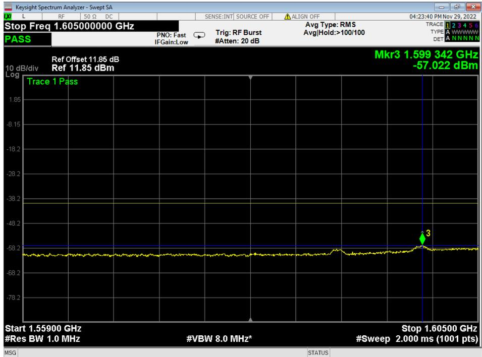
**Figure 8 – Part 25.216(c), Transmitting at 1616.020833 MHz, Conducted Measurement**
