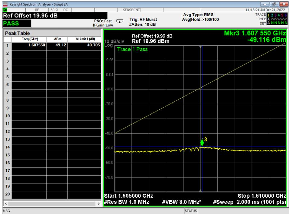
Figure 11 – Part 25.216(g), Transmitting at 1616.020833 MHz, Conducted Measurement
