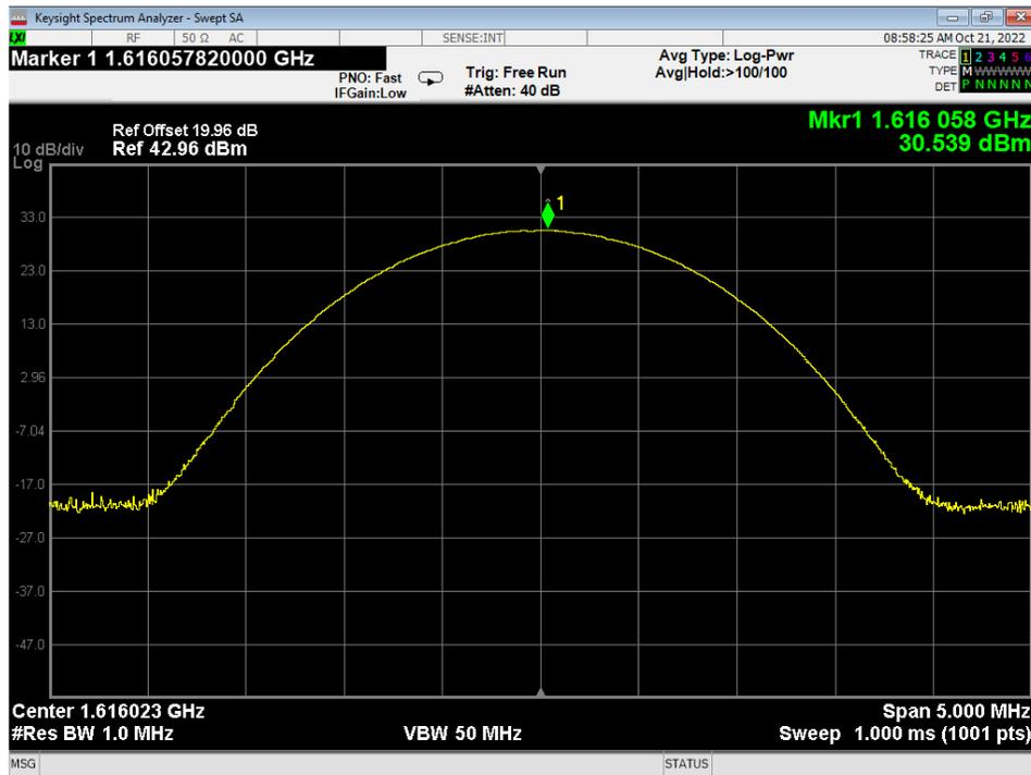
Figure 23 – Conducted Average Power Measurement, Iridium, Low
