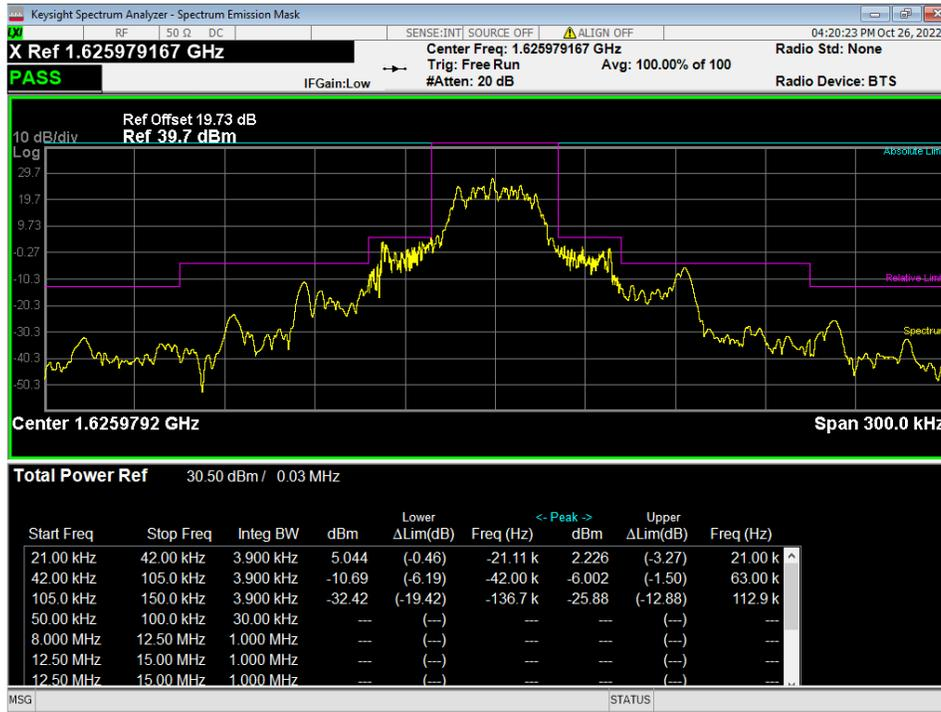
Figure 7 – Part 25.202(f) Mask, Transmitting at 1625.979167 MHz
