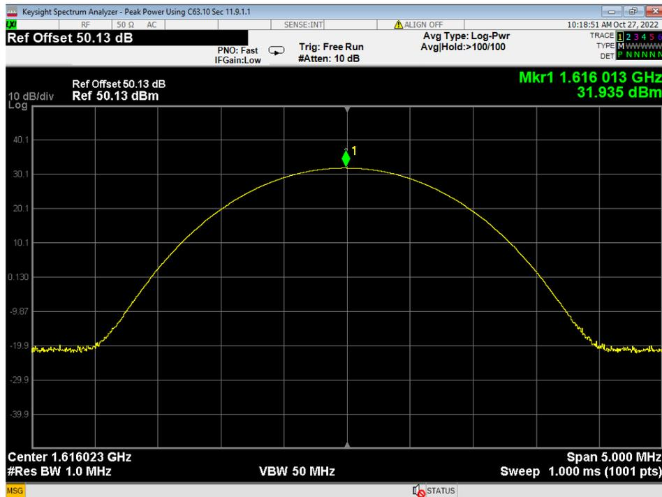
Figure 24 – Radiated Average Power Measurement, Iridium, Low
