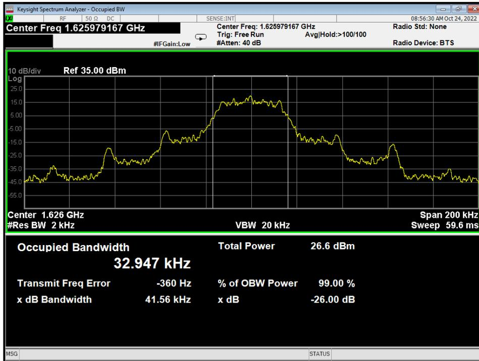
Figure 19 – Supporting Plots for modulation characteristic, High Channel
