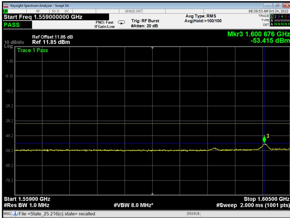
**Figure 10 – Part 25.216(c), Transmitting at 1625.979167 MHz, Conducted Measurement**
