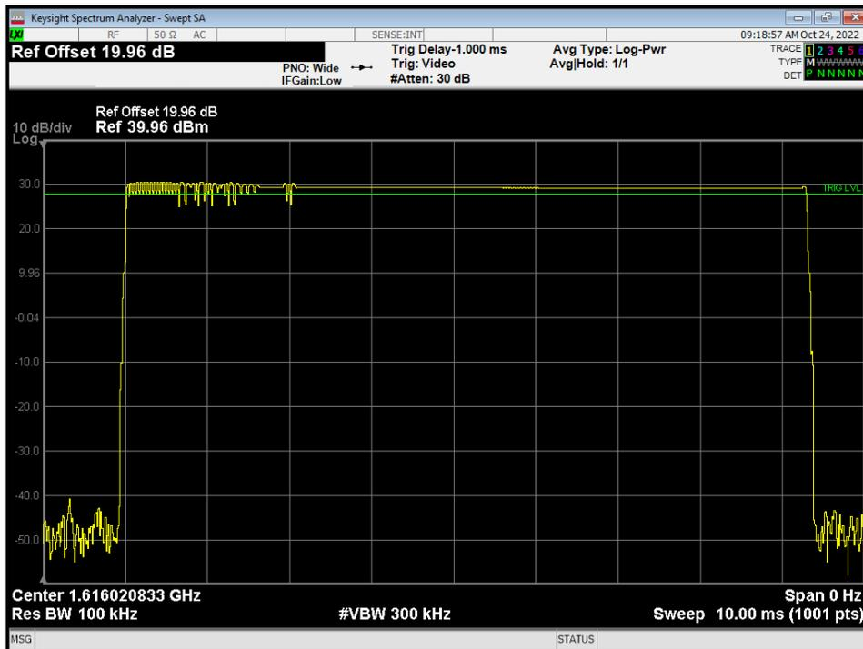
Figure 20 – Supporting Plots for modulation characteristic, Low Channel
