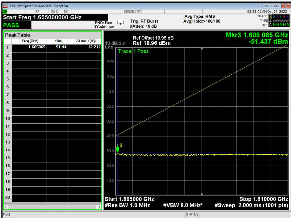
Figure 12 – Part 25.216(g), Transmitting at 1620.979167 MHz, Conducted Measurement
