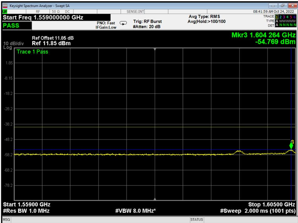
**Figure 9 – Part 25.216(c), Transmitting at 1620.979167 MHz, Conducted Measurement**
