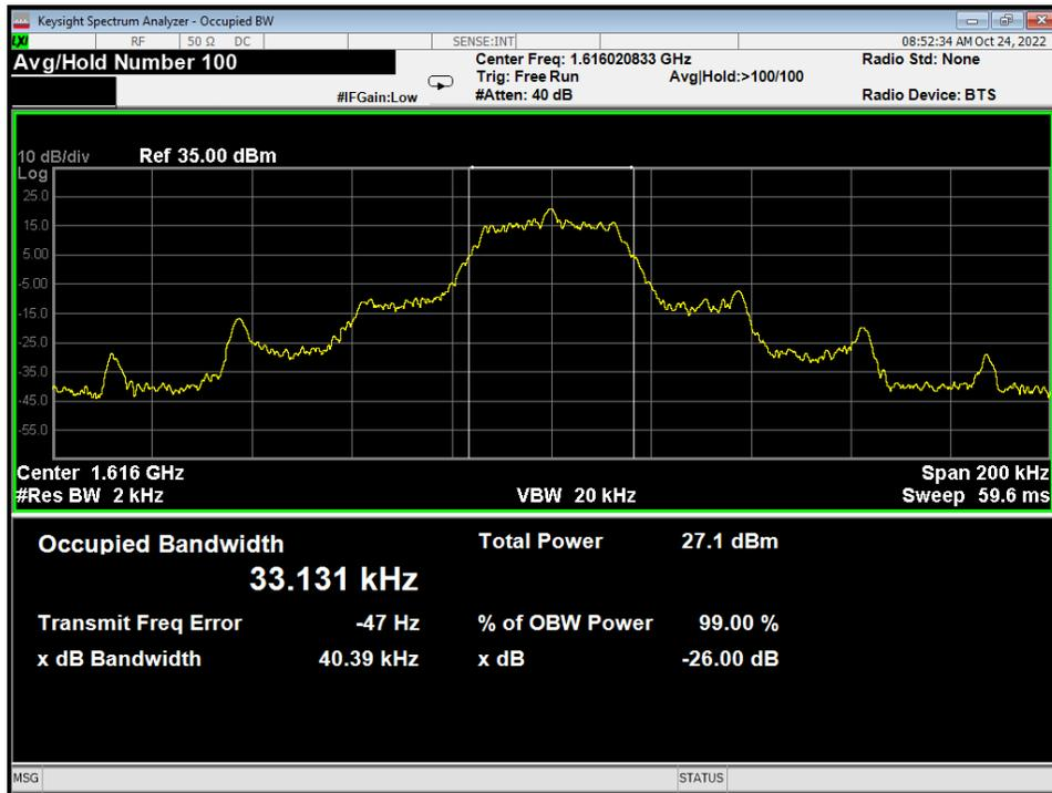
Figure 17 – Supporting Plots for modulation characteristic, Low Channel
