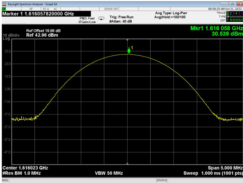
**Figure 2 – Conducted Average Output Power, Transmitting at 1616.020833 MHz**
