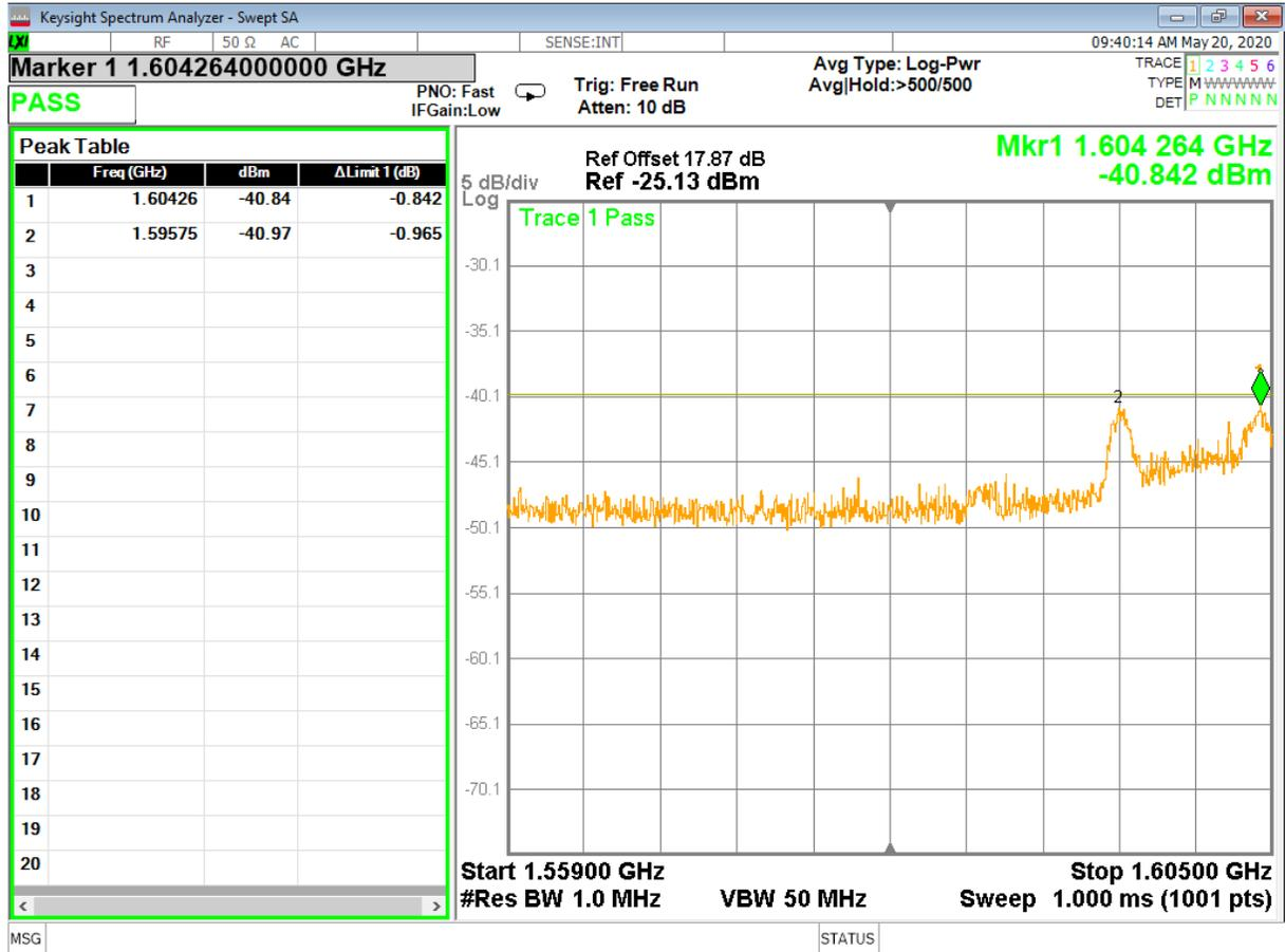
**Figure 6 – Part 25.212(c), Transmitting at 1620.979167 MHz, Conducted Measurement**
