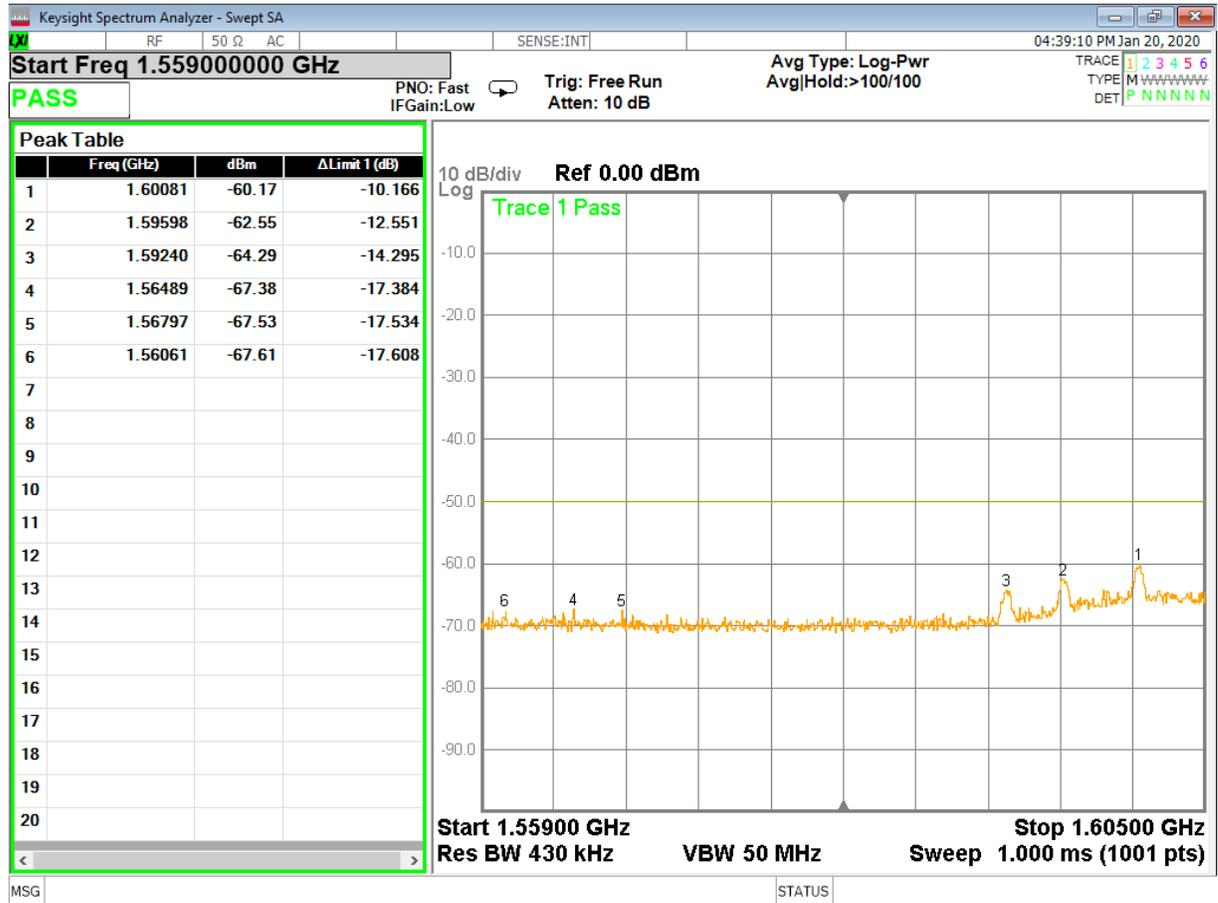
Figure 7 – Part 25.216(c), Transmitting at 1625.979167 MHz, Conducted Measurement
