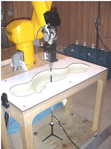
DASY 4 SAR System with SAM Phantom
