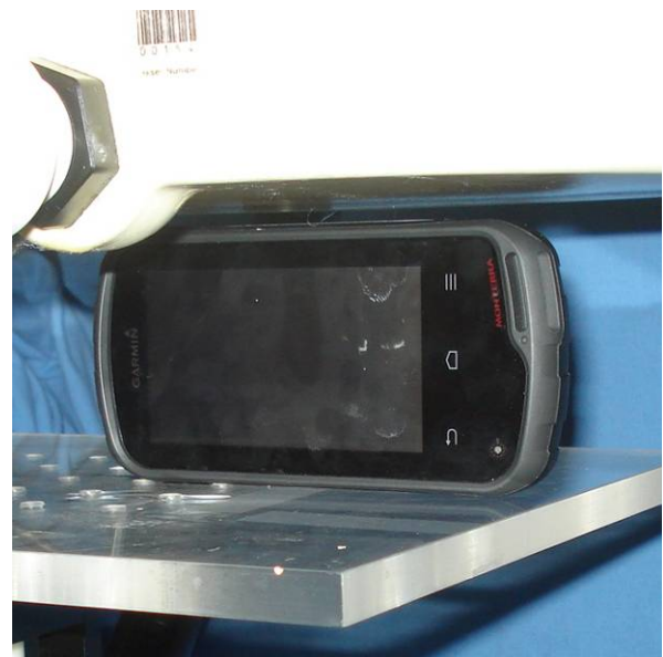
DUT side (power button side) facing phantom - 5mm spacing
