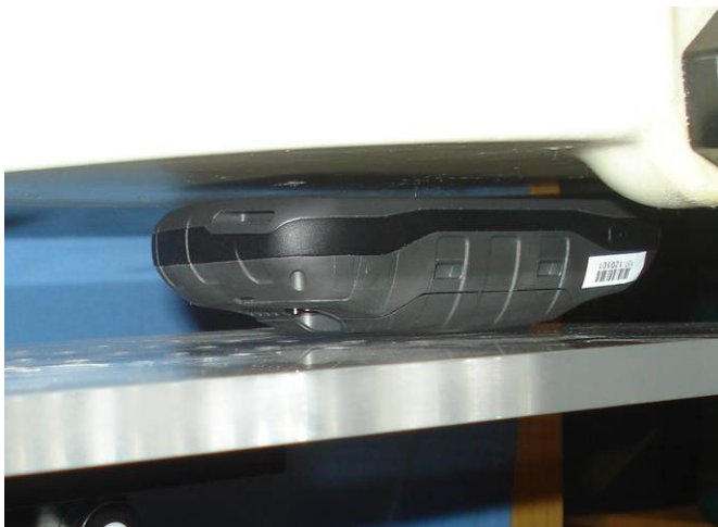
DUT front (screen side) facing phantom - 5mm spacing
