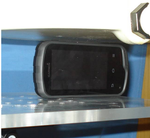
DUT side (power button side) facing phantom - 5mm spacing
