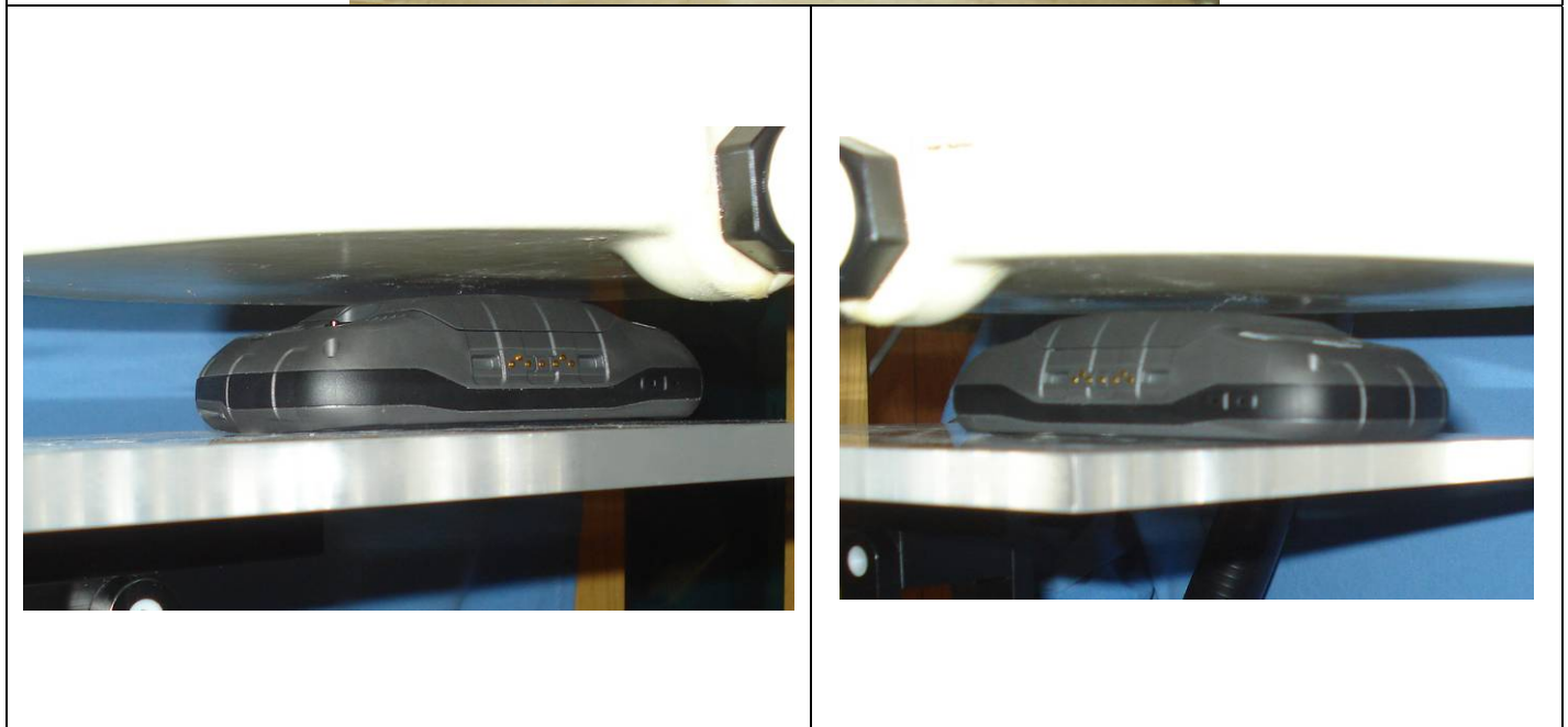
DUT back (battery side) facing phantom - 5mm spacing
