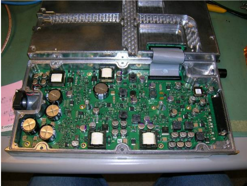
GTS8XX Internal photograph of the Power Supply board (top side)
