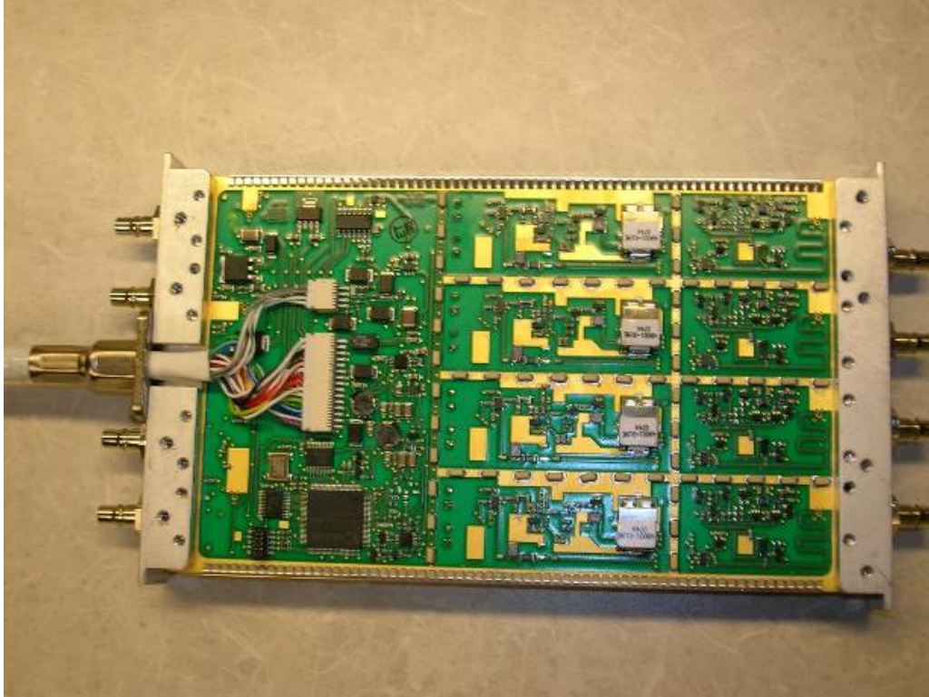
GPA65 Internal photograph of the Receiver board
