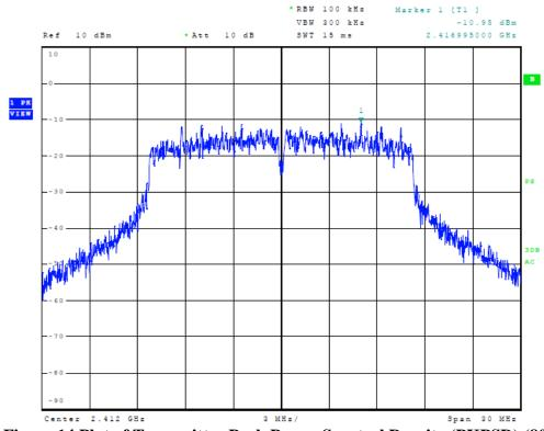
Figure 14 Plot of Transmitter Peak Power Spectral Density (PKPSD) (802.11 g-mode)
