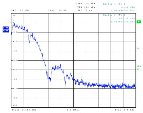
Figure 9 Plot of Upper Band Edge (802.11 b-mode)
