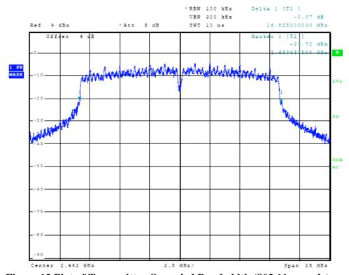
Figure 12 Plot of Transmitter Occupied Bandwidth (802.11 g-mode)
