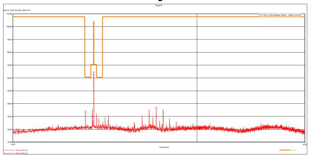
Figure 1 – NFC Radiated Emissions Plot, 10MHz – 30MHz
