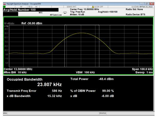
Figure 6 - NFC Occupied Bandwidth
