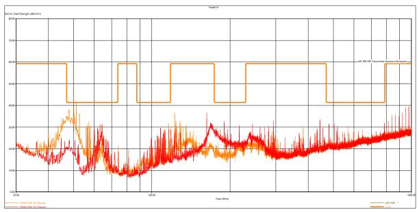
Figure 2 – NFC Radiated Emissions Plot, 30MHz – 1GHz
