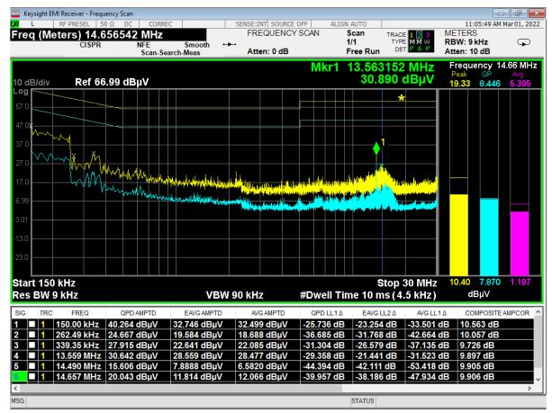
Figure 9 - Conducted Emissions Plot, Line, Idle
