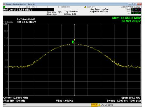
Figure 3 – NFC Field Strength Plot Corrections included
