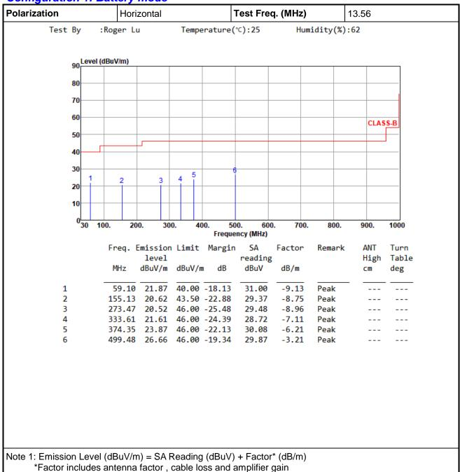
Note 2: Margin (dB) = Emission level (dBuV/m) - Limit (dBuV/m).
