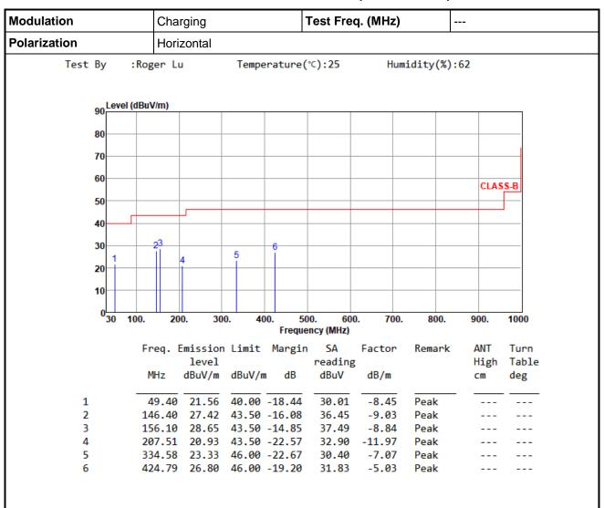
Note 1: Emission Level (dBuV/m) = SA Reading (dBuV/m) + Factor\* (dB/m)
