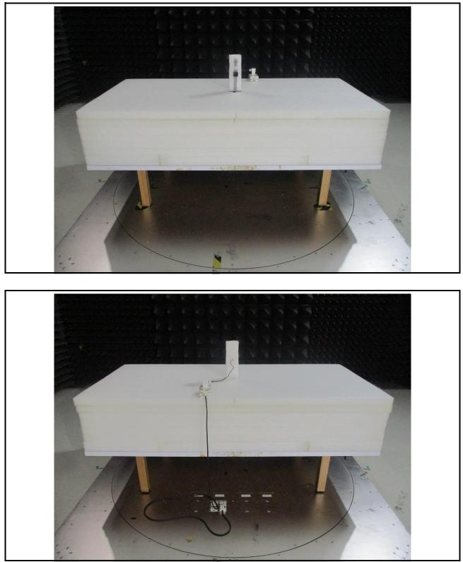
Radiated Emission Below 1GHz Test (Charger Mode)
