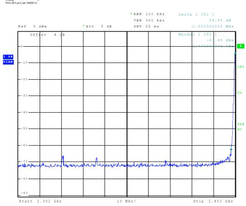
Figure 5 Plot of Transmitter Emissions Low Band Edge
