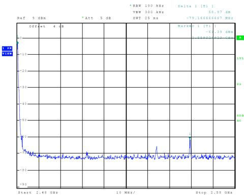
Figure 6 Plot of Transmitter Emissions High Band Edge
