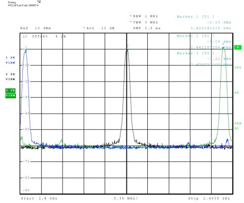
Figure 3 Plot of Transmitter Emissions Operation in 2402-2480 MHz
