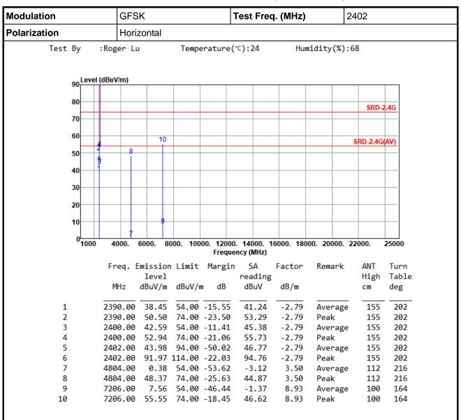
Note 1: Emission Level (dBuV/m) = SA Reading (dBuV/m) + Factor\* (dB/m)
