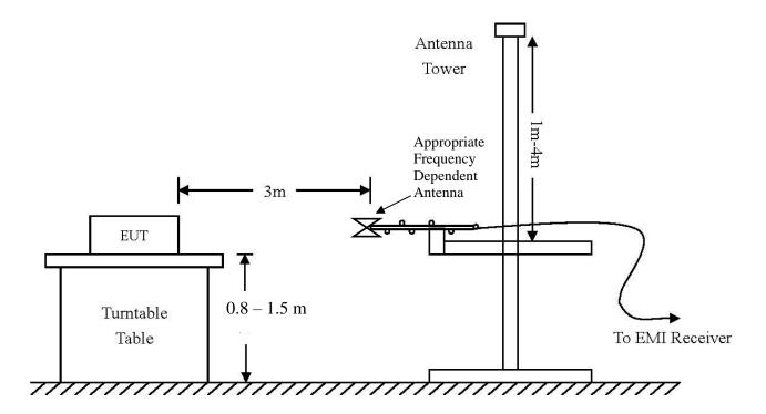
Diagram 3 Test arrangement for Antenna Port Conducted emissions
