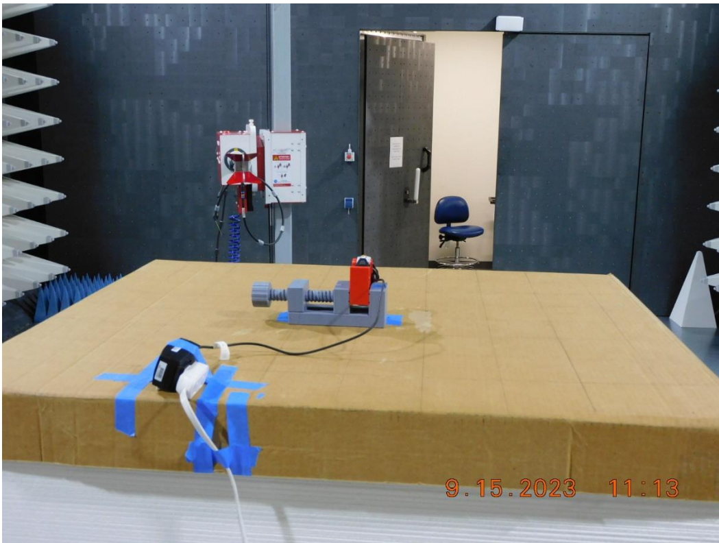
Figure RE04.8: EUT test setup Z orientation (rear view)
