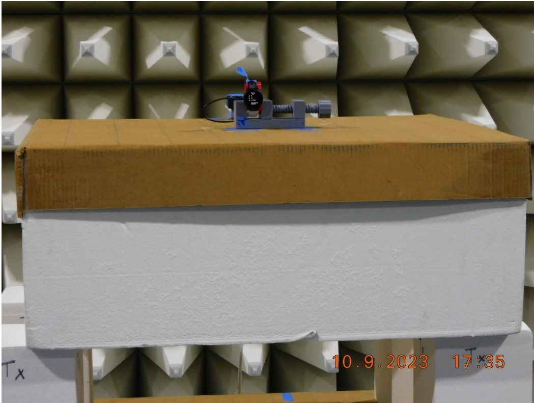
Figure RE06.5: EUT test setup, (WiFi B11 Ch1) Z orientation front view
