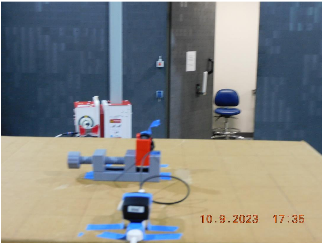
Figure RE06.6: EUT test setup, (WiFi B11 Ch1) Z orientation reverse view
