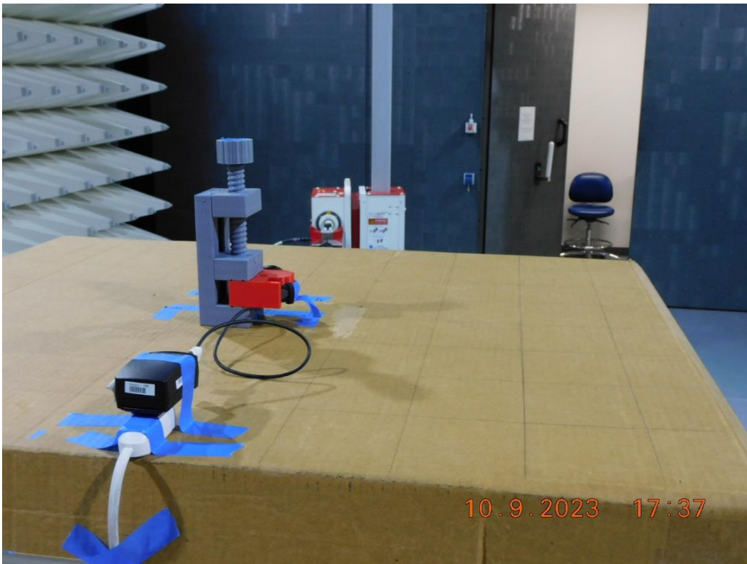
Figure RE06.8: EUT test setup, (WiFi B11 Ch6, Ch11, Ch13) X orientation reverse view
