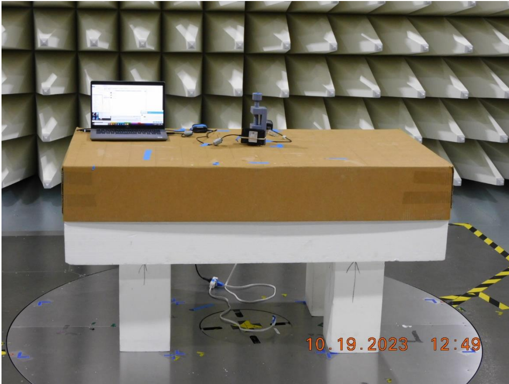
Figure RE15.2: EUT test setup, front view (X orientation)
