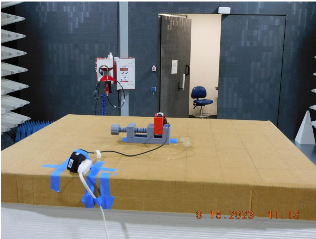
Figure RE02.6: EUT test setup Z orientation (rear view)
