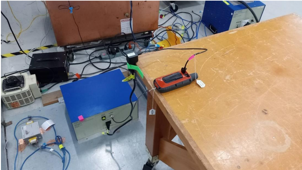
Conducted emissions test setup
