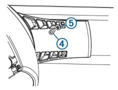
**4** Torque the hex bolts to 0.81 kgf-m (70 lfb-in. [6 lbf-ft.]) to fasten the antenna to the pedestal without damaging the antenna or the mounting hardware.
