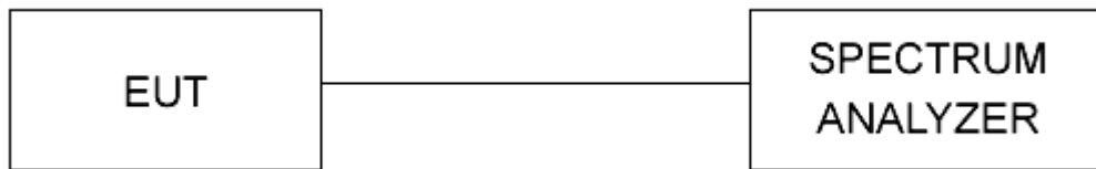
Figure 1 - Bandwidth Measurements Test Setup
