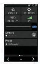
The settings widget appears. A flashing icon means the device is searching for a signal. A solid icon means the signal was found or the sensor is connected. You can select any icon to change the settings.
