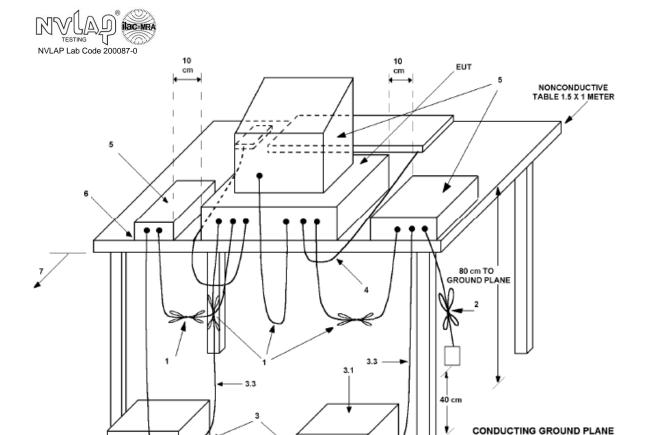
1. Interconnecting cables that hang closer than 40 cm to the ground plane were folded back and forth in the center forming a bundle 30 cm to 40 cm long.
