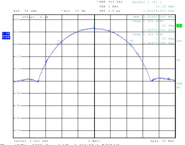
Figure 18 Plot of 99% Occupied Bandwidth Mode 5 802.11b
