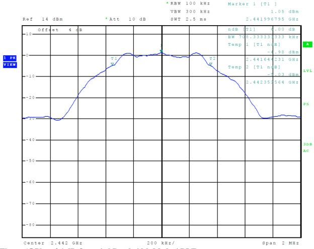
Figure 15 Plot of 6-dB Occupied Bandwidth Mode 4 BLE
