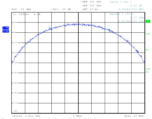
Figure 17 Plot of 6-dB Occupied Bandwidth Mode 5 802.11b
