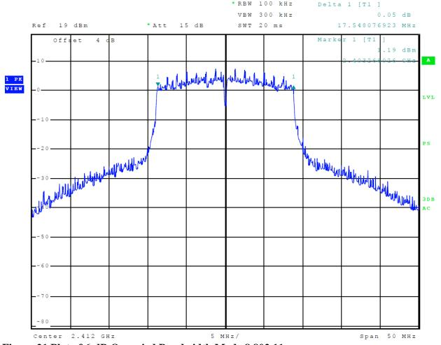
Figure 21 Plot of 6-dB Occupied Bandwidth Mode 8 802.11n
