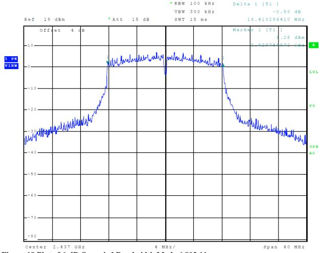
Figure 19 Plot of 6-dB Occupied Bandwidth Mode 6 802.11g
