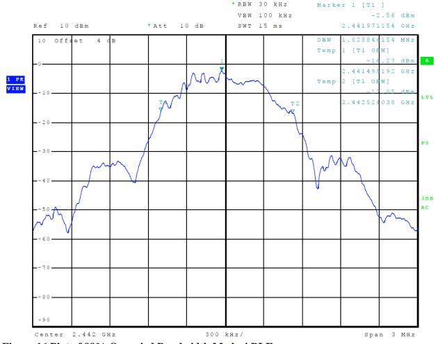
Figure 16 Plot of 99% Occupied Bandwidth Mode 4 BLE
