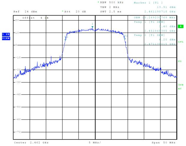
Figure 22 Plot of 99% Occupied Bandwidth Mode 9 802.11n
