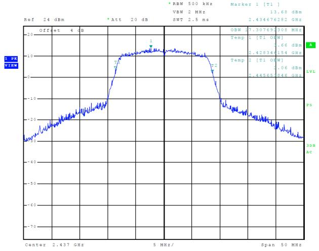
Figure 20 Plot of 99% Occupied Bandwidth Mode 7 802.11g
