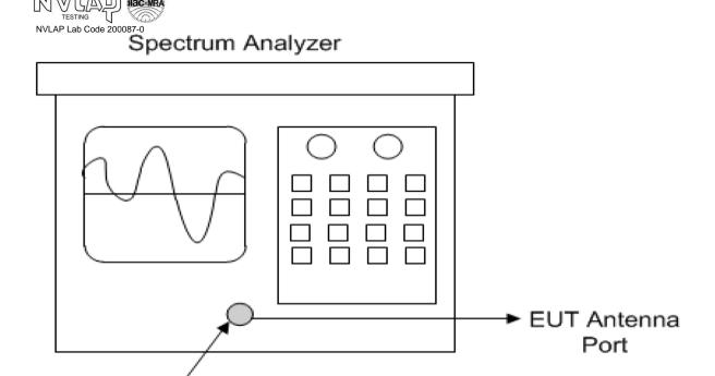
Diagram 4 Test arrangement for Antenna Port Conducted emissions
