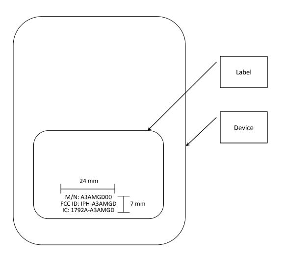
Back of device (Placed on the device behind battery door)
