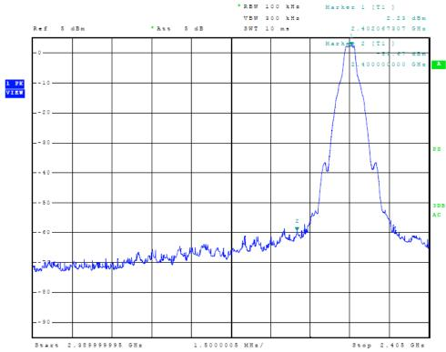
Figure Seven Plot of Lower Band Edge
