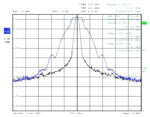
Figure Five Plot of Occupied Bandwidth
