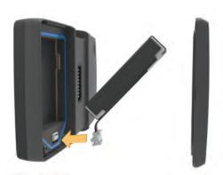
7 Replace the battery cover and tighten the screws.
