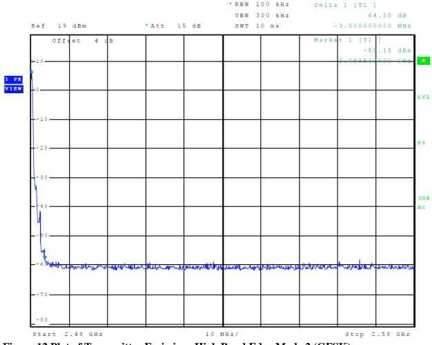
Figure 12 Plot of Transmitter Emissions High Band Edge Mode 2 (GFSK)
