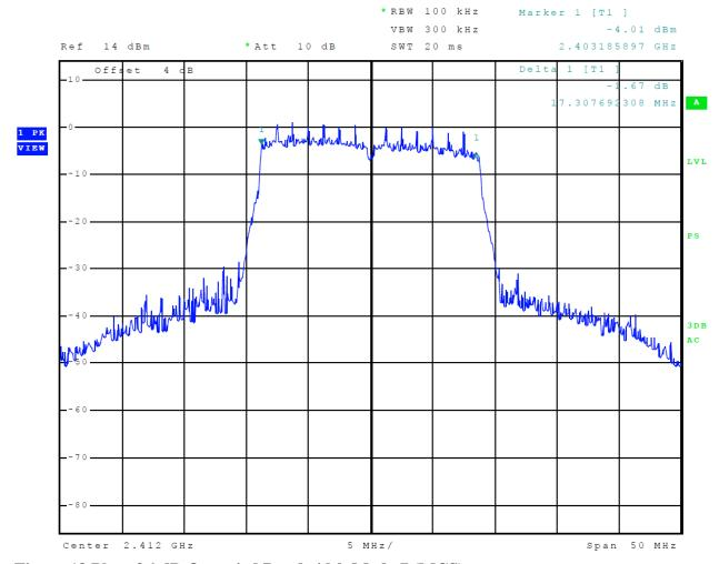
Figure 18 Plot of 6-dB Occupied Bandwidth Mode 7 (MCS)
