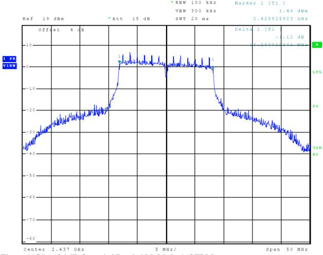
Figure 16 Plot of 6-dB Occupied Bandwidth Mode 6 (OFDM)
