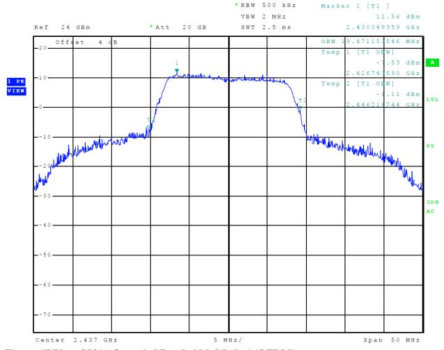
Figure 17 Plot of 99% Occupied Bandwidth Mode 6 (OFDM)
