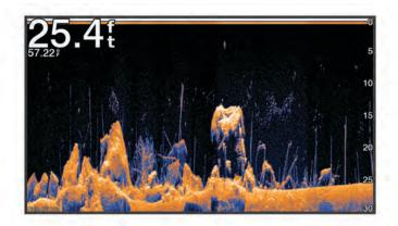
Traditional transducers emit a conical beam. The Garmin ClearVü scanning sonar technology emits two narrow beams, similar to the shape of the beam in a copying machine. These beams provide a clearer, picture-like image of what is beneath the boat.
