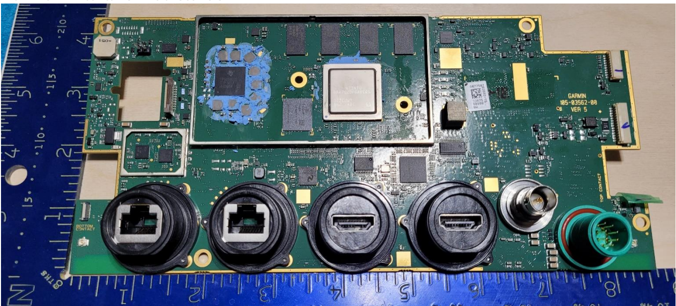
Main PCBA – contains RF transceivers
