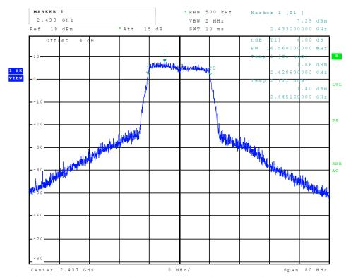
Figure 18 Plot of Transmitter 6-dB Occupied Bandwidth (802.11 g-mode)
