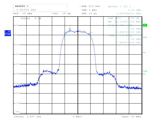
Figure 16 Plot of Transmitter 6-dB Occupied Bandwidth (802.11 b-mode)
