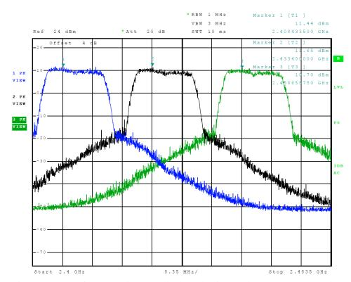
Figure 8 Plot of Transmitter Emissions in Operational Frequency (802.11 g-Mode)
