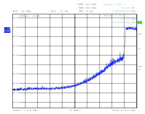
Figure 12 Plot of Lower Band Edge (802.11 n-mode)
