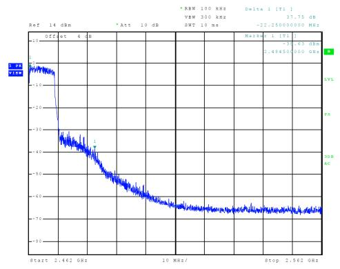
Figure 15 Plot of Upper Band Edge (802.11 n-mode)
