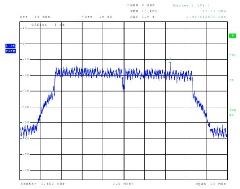
Figure 23 Plot of Transmitter Power Spectral Density (802.11 g-mode)
