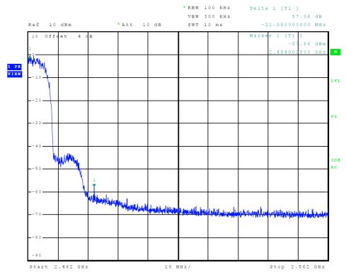
Figure 13 Plot of Upper Band Edge (802.11 b-mode)
