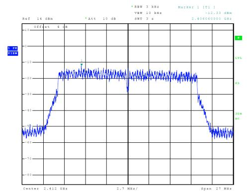
Figure 24 Plot of Transmitter Power Spectral Density (802.11 n-mode)
