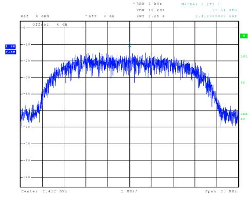
Figure 22 Plot of Transmitter Power Spectral Density (802.11 b-mode)
