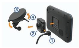
2 Press the mount ② onto the suction cup ③ until it snaps into place.
